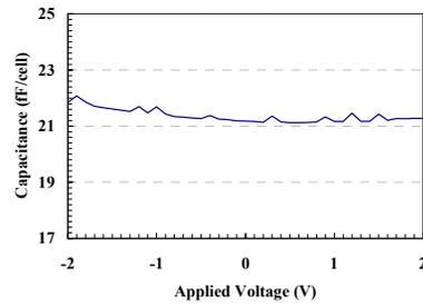
Fig. 6 CV plot of Al<sub>2</sub>O<sub>3</sub> with ALD-TiN top electrode.
