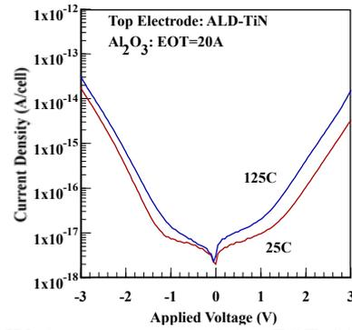
Fig. 5 IV characteristic of Al<sub>2</sub>O<sub>3</sub> (EOT=20Å) with ALD-TiN top electrode.
