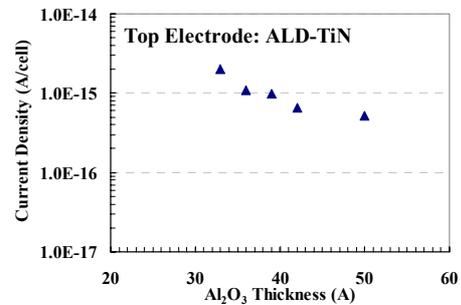
Fig. 8 Leakage current as a function of Al<sub>2</sub>O<sub>3</sub> thickness.
