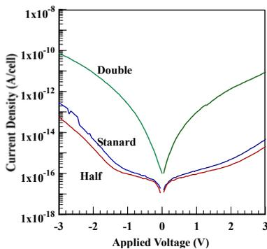
Fig. 4 The effect of plasma amount for MOCVD-TiN on leakage current.
