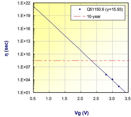
Fig. 7 Results of TDDDB Measurements.
