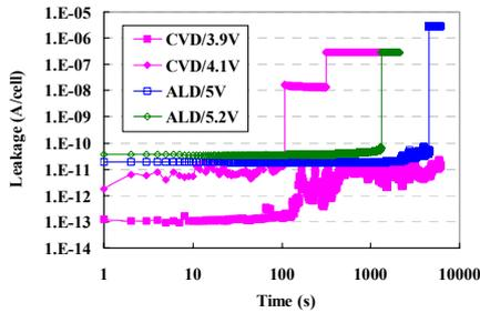
Fig. 3 The effect of top electrode on I-t measurement.
