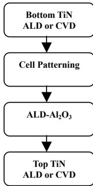
Fig. 1 Process flow of Al<sub>2</sub>O<sub>3</sub>-MIM capacitors.
