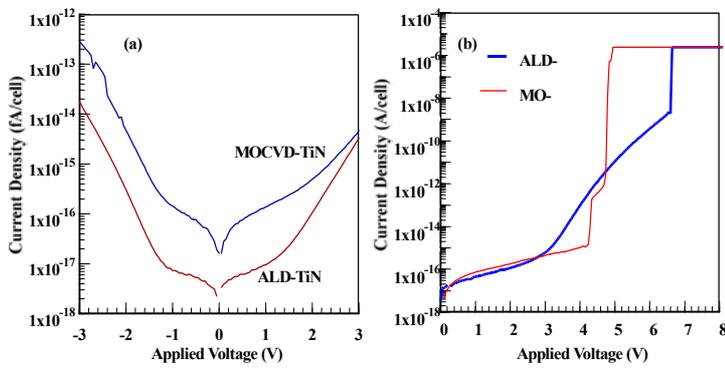
Fig. 2 The effect of top electrode on (a) leakage and (b) breakdown voltage.
