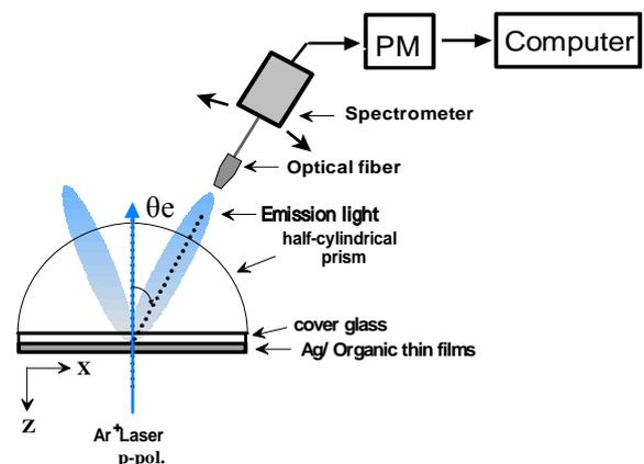
Fig.1 Kretschmann configuration and a system for detecting emission light in the reverse irradiation.
