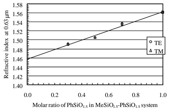
Fig. 1 Index dependence on phenyl contents in the film for TE and TM polarization at a wavelength of 0.63μm.
