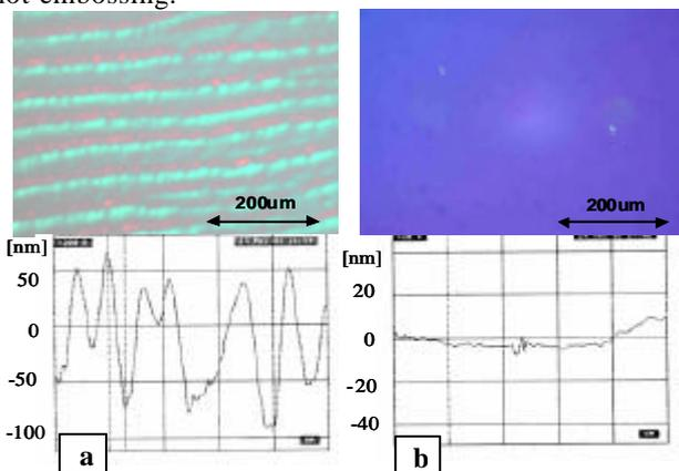
Fig. 3 Nomarski micrograph and surface profile of non-planarized (a) and planarized (b) waveguides. Profiling length was 500 $\mu$ m.
