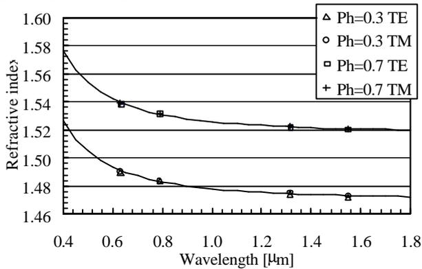
Fig. 2 Index of the phenyl-methyl silsesquioxane film for TE and TM modes as a function of wavelength.
