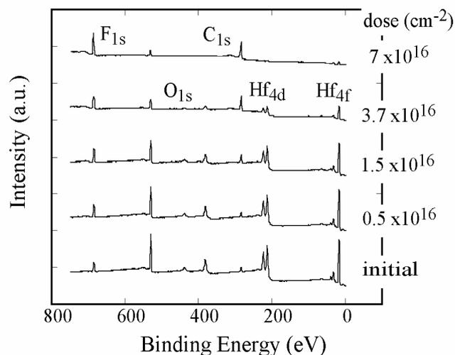
**Fig.5** Series of XPS spectra of  $HfO_2$  surfaces after each dose of  $CF^+$  ion irradiation with energy of 1000 eV.
