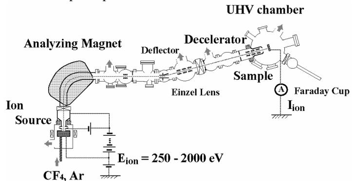
Fig.1 Schematic diagram of mass-analyzed low-energy ion-beam apparatus.
