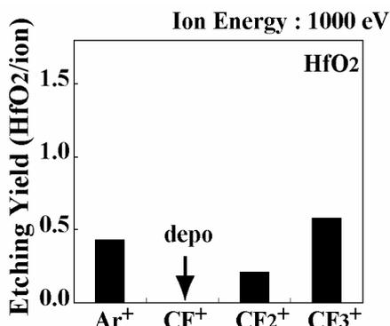
**Fig.2** Etching yields of  $HfO_2$  for  $Ar^+$  and  $CF_x^+$  ( $X=1, 2, 3$ ) ion with energy of 1000 eV.
