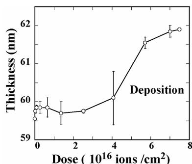
**Fig.4** Change in thickness of irradiated  $HfO_2$  film as a function of  $CF^+$  ion dose with energy of 1000 eV.
