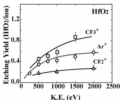
**Fig.3** Etching yields of  $HfO_2$  as a function of ion energy
