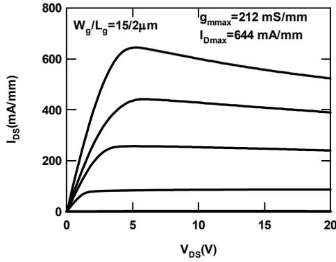
Fig. 4. Typical  $I_{DS}$ - $V_{DS}$  characteristics of AlGaIn/GaN HEMTs  $V_G=+1.5V$ ,  $\Delta V_G=-1.0V$
