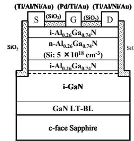
Fig. 1. Schematic diagram of fabricated AlGaIn/GaN HEMTs
