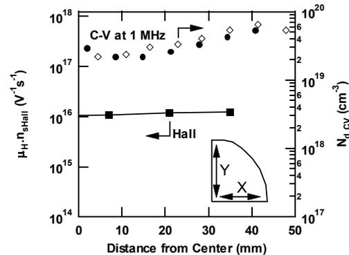
Fig. 3. Line scan distribution of the product of  $\mu_{H} \cdot n_{\text{Hall}}$  and  $N_{\text{dcv}}$  for AlGaIn/GaN HEMTs
