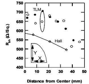
Fig. 2. Line scan distribution of  $R_{sh}$  measured from Hall and TLM method
