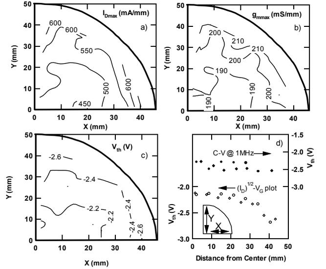
Fig. 5. Contour mapping of a)  $I_{Dmax}$ , b)  $g_{mmax}$ , and c)  $V_{th}$  of AlGaIn/GaN HEMTs on a quarter of 100-mm diameter sapphire. d) Line scan distribution of  $V_{th}$  measured from C-V and  $(I_b)^{1/2} - V_G$  plot.
