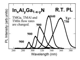
Fig. 1 Photoluminescence (PL) spectra measured at room temperature from quaternary In<sub>x</sub>Al<sub>y</sub>Ga<sub>1-x-y</sub>N grown with various growth conditions.
