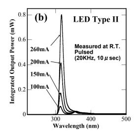
Fig. 3 Integrated output power for (a) LED I and (b) LED II measured under pulsed current injection at room temperature.
