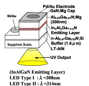
Fig. 2 Schematic structure of UV-LED with quaternary InAlGaN emitting region.
