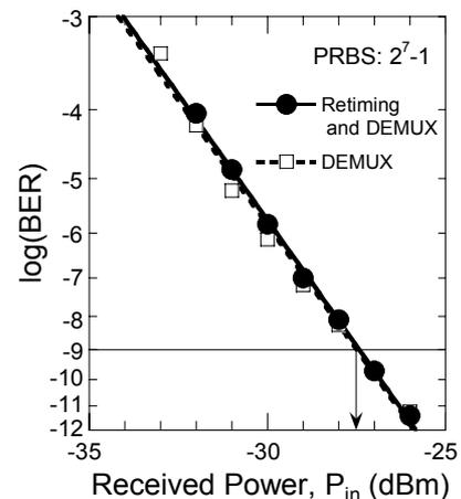
Fig. 4 Bit error rate curves after demultiplexing.
