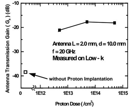
Fig. 9 Antenna transmission gain ( $G_a$ ) versus proton dose. (Antenna  $L=2.0 \text{ mm}$ ,  $d=10.0 \text{ mm}$ )
