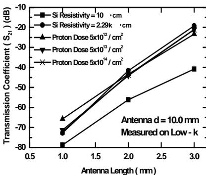
Fig. 10 Transmission coefficient versus Antenna length. (Effect of proton dose) (Antenna  $d=10.0 \text{ mm}$ )
