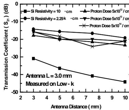
Fig. 11 Transmission coefficient versus Antenna Distance. (Effect of proton dose) (Antenna  $L=3.0 \text{ mm}$ )
