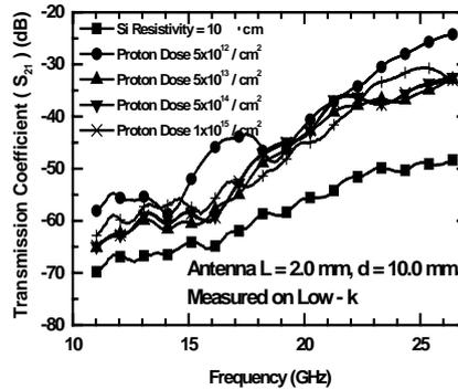
Fig. 8 Transmission coefficient ( $S_{21}$ ) versus frequency. (Effect of proton dose) (Antenna  $L=2.0 \text{ mm}$ ,  $d=10.0 \text{ mm}$ )
