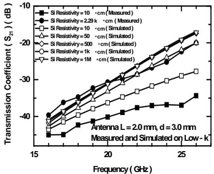
Fig. 12 Transmission coefficient versus frequency with Si resistivity as a parameter. Measured and simulated data are compared. (Antenna  $L=2.0 \text{ mm}$ ,  $d=3.0 \text{ mm}$ )
