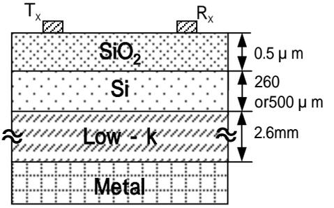
Fig. 3. Schematic cross-sectional diagram of dipole transmitter-receiver antennas.  $T_x$  = Transmitter,  $R_x$  = Receiver.
