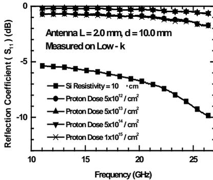
Fig. 7 Reflection coefficient ( $S_{11}$ ) versus frequency. (Effect of proton dose) (Antenna  $L=2.0 \text{ mm}$ ,  $d=10.0 \text{ mm}$ )
