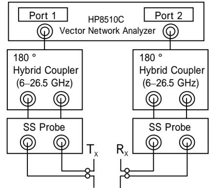
Fig. 6. Experimental set-up for on chip antenna characterization.
