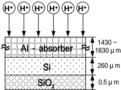
Fig. 4. Schematic diagram of proton implantation.
