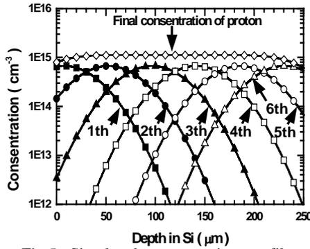
Fig. 5. Simulated concentration profile of proton in Si. Implantation was done in 6 steps with a fixed energy of 17.4 MeV and a fixed dose of  $10^{15} \text{ cm}^{-2}$ .
