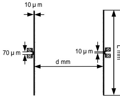
Fig. 2. A plan-view of transmitting and receiving antennas on a Si substrate.
