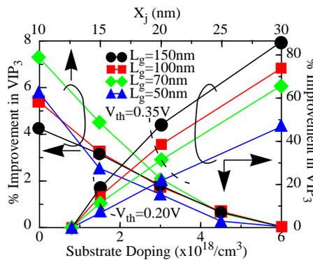
Fig. 5: Percentage change in  $VIP_3$  with increase in  $N_A$  and decrease in  $X_j$ .  $VIP_3$  values at  $N_A=8 \times 10^{17}$  and  $X_j=30nm$  are used to calculate corresponding percentage changes. Dotted lines show the constant  $V_{th}$  devices.
