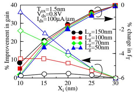
Fig. 6: Percentage change in gain and  $f_T$  with decrease in  $X_j$ . Gain and  $f_T$  values corresponding to  $X_j=30nm$  are used as base values for calculating the percentage changes.
