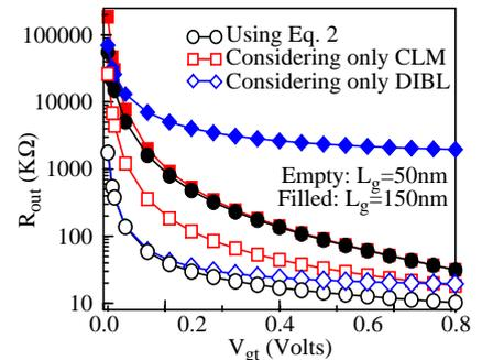
Fig. 2: CLM and DIBL components of  $R_{out}$ .
