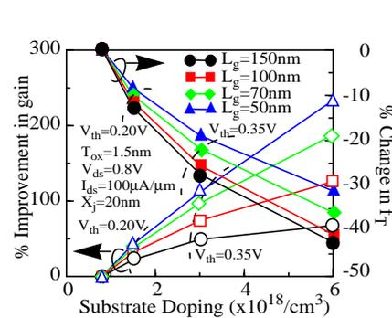
Fig. 4: Percentage change in gain and  $f_T$  with increase in substrate doping. Gain and  $f_T$  values corresponding to  $N_A=8 \times 10^{17}$  are used as base values for calculating the percentage changes. Dotted lines show the constant  $V_{th}$  devices.
