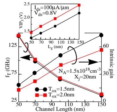
Fig. 3: Gain,  $f_T$  and  $VIP_3$  (inset) vs.  $L_g$  for  $T_{ox}=1.5$  and  $2nm$ .
