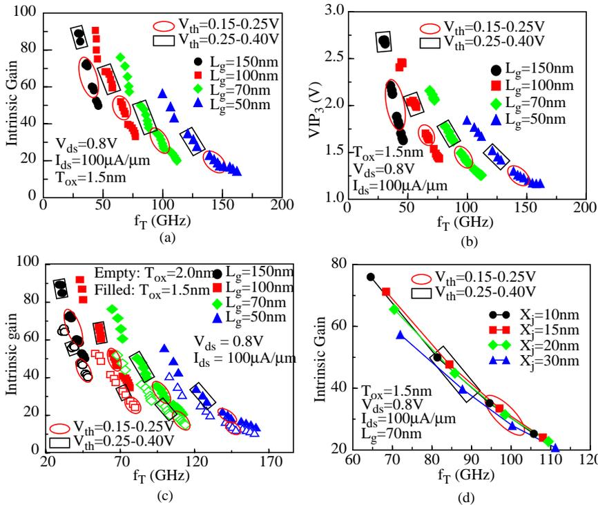
Fig. 1: (a) gain vs.  $f_T$  and (b)  $VIP_3$  vs.  $f_T$  trade-offs for various channel lengths. Impact of (c)  $T_{ox}$  and (d)  $X_j$  on gain vs.  $f_T$  trade offs. In (a), (b) and (c)  $N_A$  as well as  $X_j$  are varied for a given  $L_g$  and  $T_{ox}$  to obtain various points. In (d) only  $N_A$  is varied for a given  $X_j$ , to obtain the trade-off curves.
