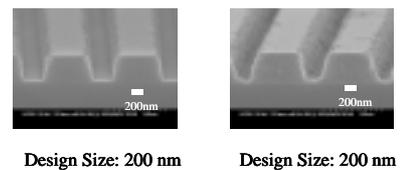
Fig. 8. SEM micrographs of photosensitive MSQ without porogen (a) (left hand side) and with 10 wt% porogen (b) (right hand side): (electron-beam exposure dose :  $9.0 \mu\text{C}/\text{cm}^2$ ,  $L/S=1:5$ )
