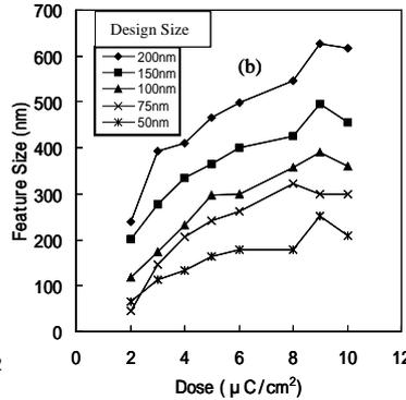
Fig. 6. Characteristic curves for photosensitive porous MSQ (10 wt% porogen) in electron-beam lithography: (a) exposure depth versus exposure dose, (b) feature size versus exposure dose.
