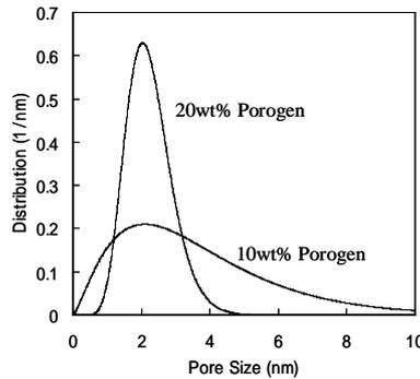
Fig. 4. Pore size distribution measured by X-ray scattering measurement.
