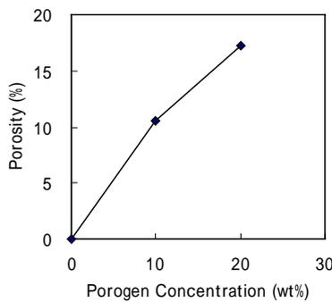
Fig. 3. Calculated porosity versus porogen concentration from measured refractive index.
