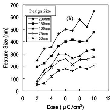
Fig. 7. Characteristic curves for photosensitive MSQ without porogen in electron-beam lithography: (a) exposure depth versus exposure dose, (b) feature size versus exposure dose.
