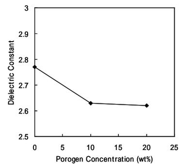
Fig. 5. Dielectric constants versus porogen concentration for photosensitive porous MSQ.
