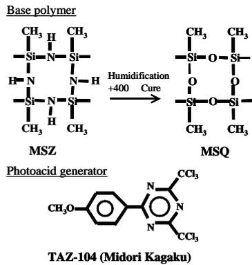
Fig. 1. Schematic diagrams of MSZ and MSQ, and photoacid generator.
