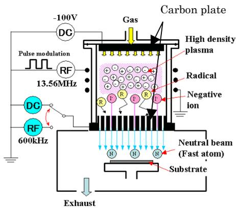
Fig. 1 Neutral beam etching system.
