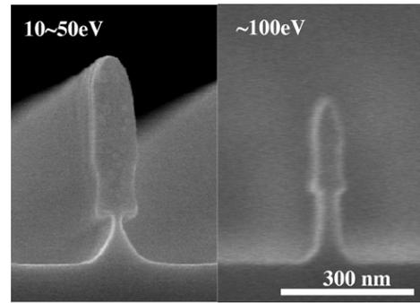
Fig. 2 Pattern profiles of poly-Si etched at different bias conditions in a pure SF<sub>6</sub> gas system.
