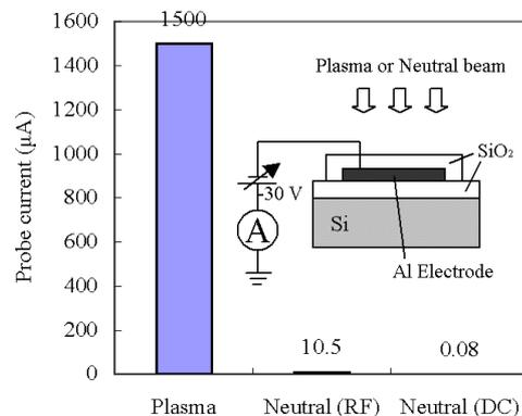
Fig. 5 Probe current of the on-wafer monitoring device irradiated by SF<sub>6</sub> plasma or neutral beam.
