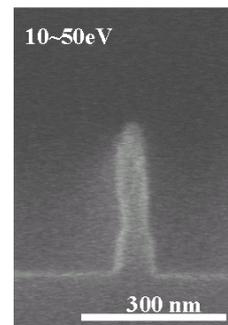
Fig. 3 Pattern profiles of poly-Si etched in a pure Cl<sub>2</sub> gas system.
