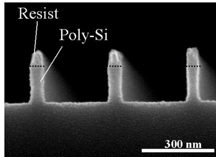
Fig. 4 Pattern profile of poly-Si etched at an optimum gas ratio in a Cl<sub>2</sub>/SF<sub>6</sub> gas system.
