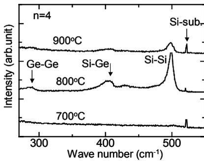
Fig.3 Raman spectra for samples (n=4) annealed at 700, 800, and  $900^\circ\text{C}$  for 30min.
