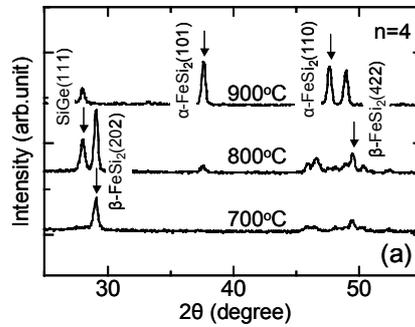
Fig.4 XRD spectra for samples (n=4) annealed at 700, 800, and  $900^\circ\text{C}$  for 30min (a), and lattice strain of  $\beta\text{-FeSi}_2(\text{Ge})$  as a function of n (b). In analysis of strains,  $b=c$  was assumed.
