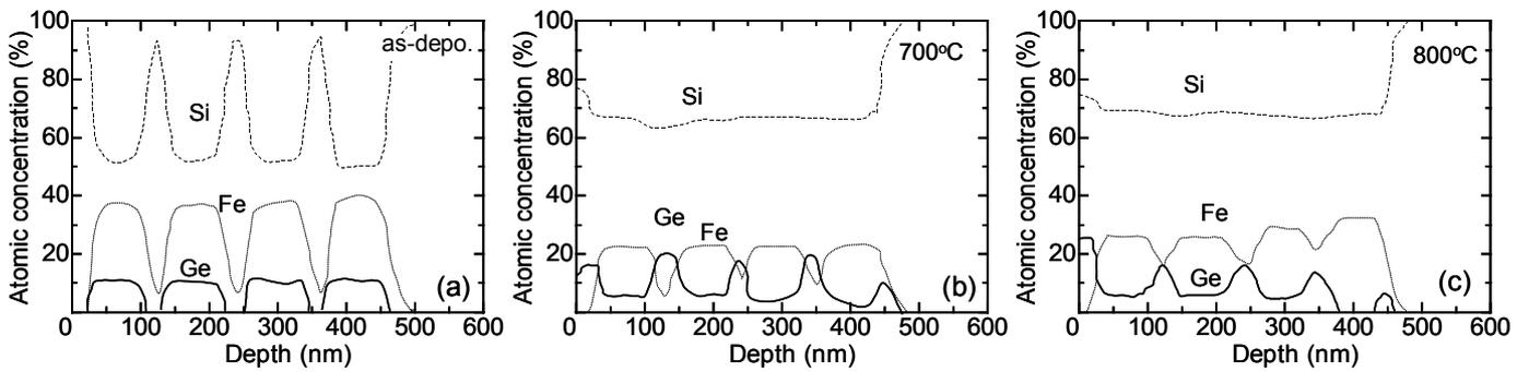
Fig.2 Concentration profiles of Fe, Si, and Ge for samples (n=4) before (a) and after annealing at 700 (b) and  $800^\circ\text{C}$  (c) for 30min.
