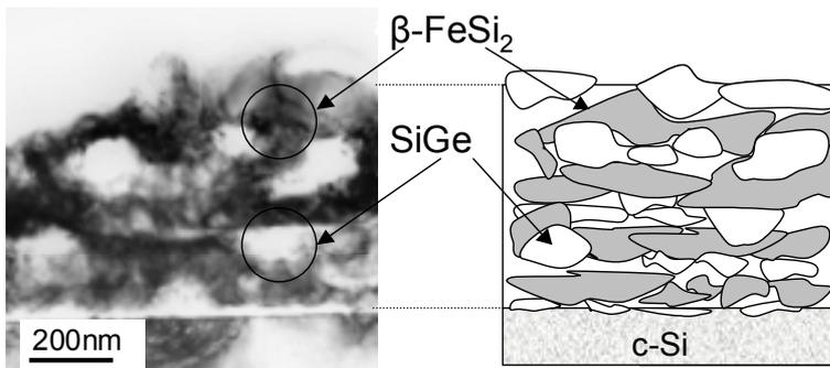
Fig.5 TEM image (a) and its schematics (b) for sample (n=4) annealed at  $800^\circ\text{C}$  for 30min.
