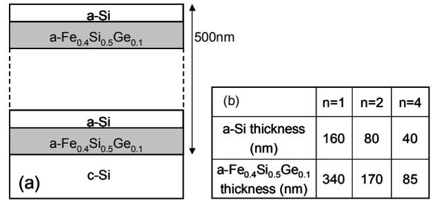
Fig.1 Schematic structure (a) and thickness parameters of samples (b).
