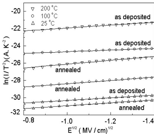
Fig. 5 The  $\ln(I/T^2)$  vs  $E^{1/2}$  plot for as-deposited and annealed ZrO<sub>2</sub> films at different temperature.
