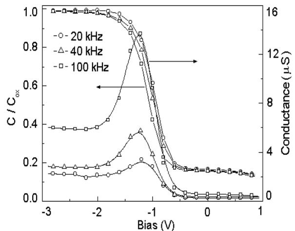
Fig. 2 Frequency dispersion in C-V and G-V characteristics.
