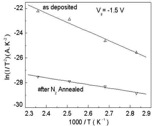
Fig. 6 The  $\ln(I/T^2)$  vs  $1000/T$  plot for as-deposited and annealed ZrO<sub>2</sub> films.
