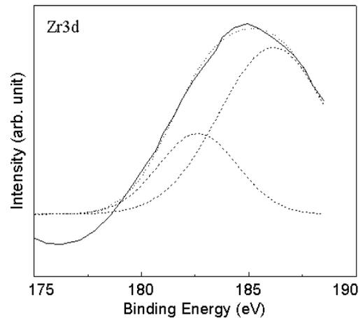
Fig. 1 Deconvoluted Zr 3d spectra for the as-deposited ZrO<sub>2</sub> films on strained Si<sub>1-y</sub>C<sub>y</sub> layers.
