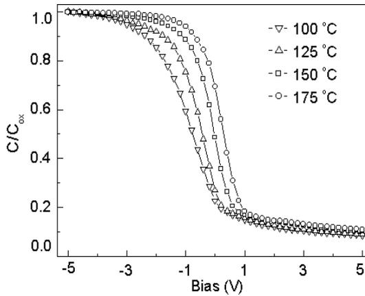
Fig. 3 C-V characteristics of ZrO<sub>2</sub> films.
