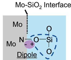
Fig.8 Electrical dipole model to explain workfunction shift at the Mo/SiO<sub>2</sub> interface.
