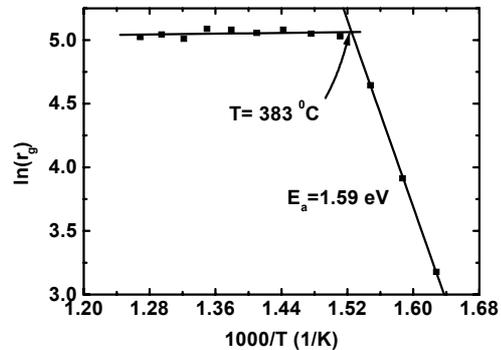
Fig. 2. Dependence of growth rate on growth temperature.
