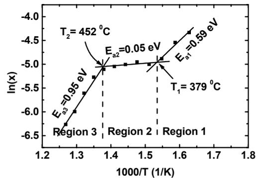
Fig. 1. Dependence of nitrogen composition on growth temperature.
