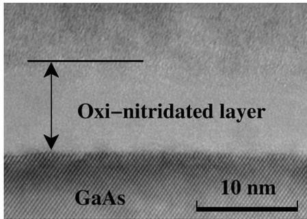
Fig. 1 Cross-sectional TEM image of the oxi-nitridated GaAs layer formed by 8hrs nitridation after 8hrs oxidation
