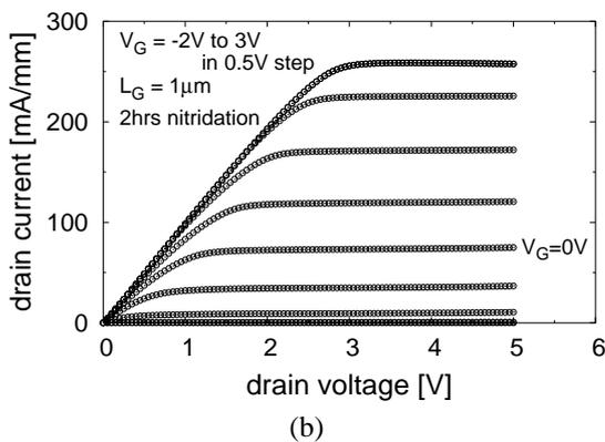
Fig. 3 Normalized DC characteristics of  $1 \mu\text{m}$  GaAs-MISFET with 4hrs oxidation (a), 2hrs nitridation after 4hrs oxidation (b).
