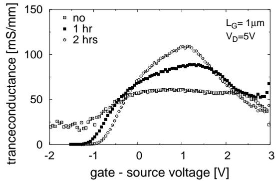
Fig. 5 Transconductans with different nitridation time at drain voltage of 5V
