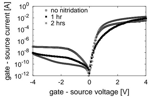
Fig. 4 MIS diode characteristics
