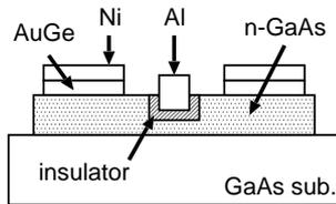
Fig. 2 Structure of GaAs-MISFET,  $N_D = 3.0 \times 10^{17} \text{ cm}^{-3}$ , thickness of channel is  $0.18 \mu\text{m}$ .
