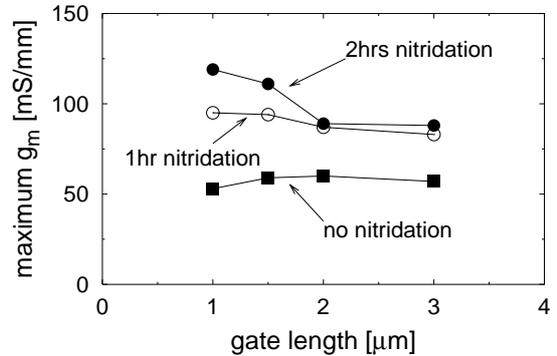
Fig. 6 Gate length dependence of maximum transconductans with different nitridation time
