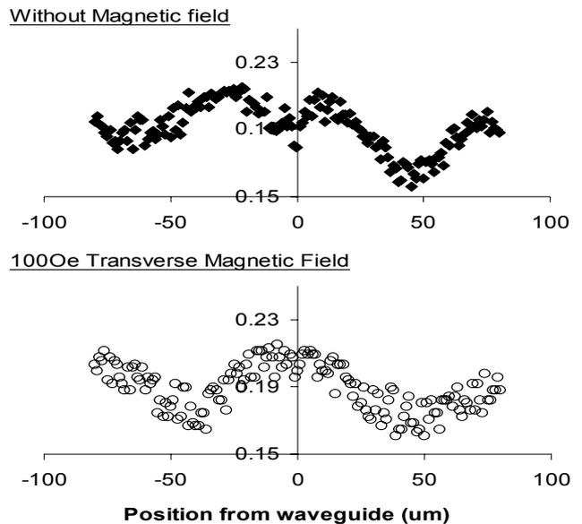
Fig. 3 Polarization dependent optical power measured by transverse scanning of waveguide without (above) and with (below) the application of external field.
