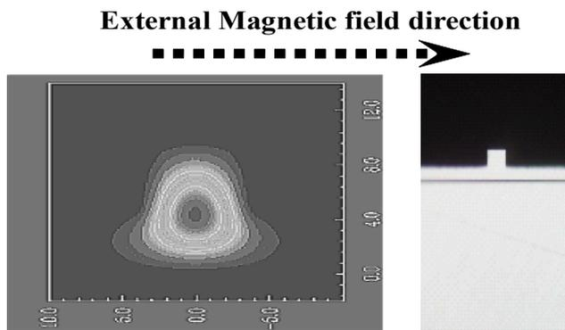
Fig. 1 Rib waveguide BPM mode cross sectional profile on the left and fabricated waveguide image on the right. The arrow indicates positive applied external magnetic field direction.
