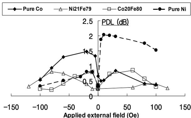
Fig. 2 In-situ polarization dependent loss measured under applied external field with different ferromagnetic overlays. Solid points represent pure metal and hollow points showing metal alloys. Dash line represents negative magnetostrictive behavior.
