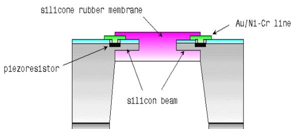
Proposed differential pressure sensor has been fabricated on the selectively diffused (100) oriented n+/n silicon substrates by unique silicon micro machining technique using porous silicon etching. Fabrication process of the differential pressure sensor is shown in Figure 2. Porous
