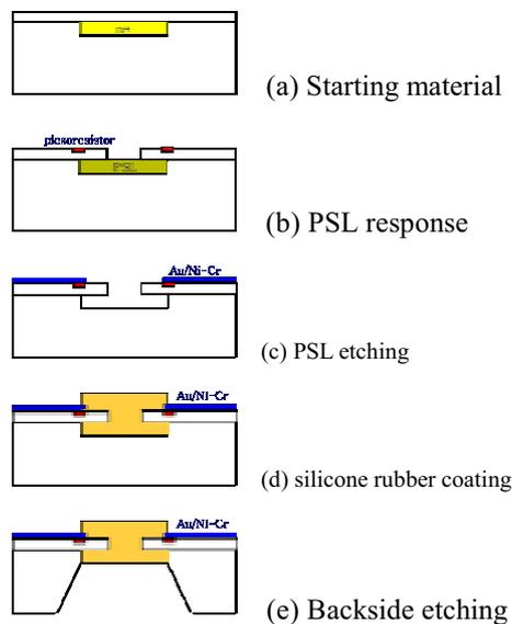
Fabricated sensors consist of a silicone rubber membrane, four silicon beams embedded in a silicone rubber membrane, four piezoresistors located on the beams, and four fixed resistors near the beams.
