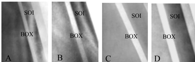
Fig. 1 XTEM micrographs of wafers implanted with  $2.5 \times 10^{17} \text{ cm}^{-2}$  at 70 keV (A),  $3.5 \times 10^{17} \text{ cm}^{-2}$  at 100 keV (B),  $4.5 \times 10^{17} \text{ cm}^{-2}$  at 130 keV (C),  $4.8 \times 10^{17} \text{ cm}^{-2}$  at 140 keV (D).
