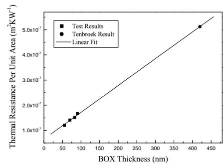
Fig. 5 Measured thermal resistance per unit area of the BOX layers with different BOX thicknesses.
