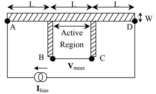
Fig. 2 Layout of the four-terminal resistor
