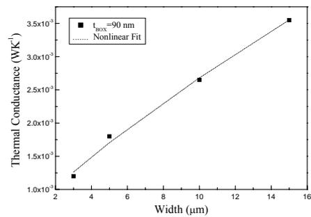
Fig. 4 Measured total thermal conductance with different widths and the nonlinear fitting result.
