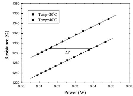
Fig. 3 Measured electrical resistance with increased power dissipation. The thickness of BOX is 90 nm.
