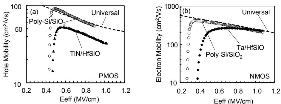
Fig. 6 Hole(a) and electron(b) mobilities of MG/HfSiO and poly-Si/SO<sub>2</sub> transistors.
