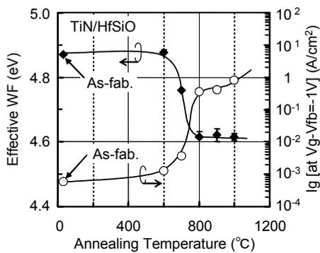
Fig. 3 Thermal stabilities of effective WF and Ig for TiN/HfSiO.
