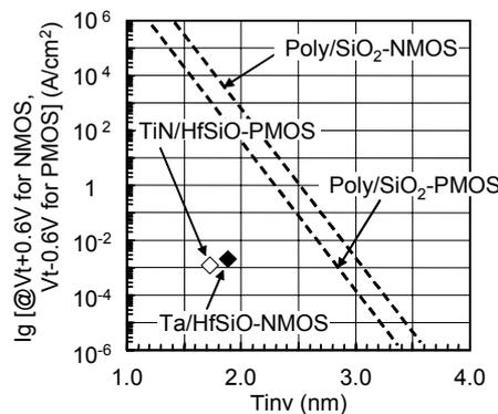
Fig. 4 Ig-Tinv characteristics of Ta and TiN gate transistors.
