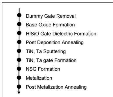
Fig. 1 Process flow of replacement gate transistor fabrication.
