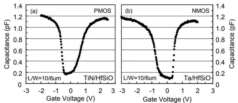
Fig. 2 C-V characteristics of MG/HfSiO-PMOS(a) and -NMOS(b) capacitors. EOT of HfSiO was 1.4 nm.
