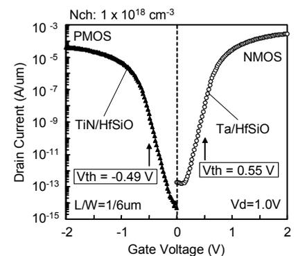
Fig. 5 Id-Vg characteristics of Ta-NMOS and TiN-PMOS transistors.
