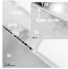
Fig. 2: TEM after gate etching: no out-of-gate Si consumption. Insert: zoom at gate edge.
