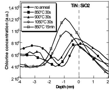
Fig. 9: SIMS profile of Chlorine in CVD TiN for different thermal budgets.
