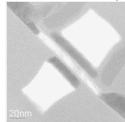
Fig. 6: TEM of 50nm gate length DG MOS with poly-TiN metal gates and NiSi salicided raised S/D.
