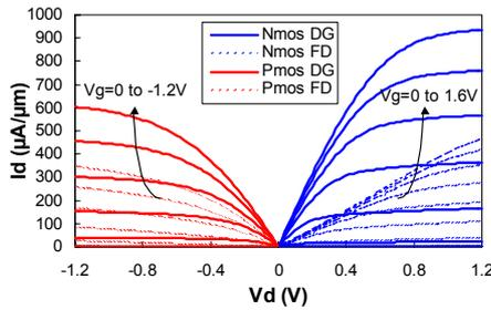
Fig. 11: Output characteristics of 40nm drawn gate length DG and FD transistors.
