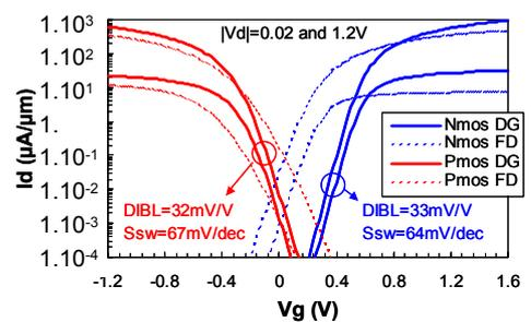
Fig. 12: Transfer characteristics of 40nm drawn gate length DG and FD transistors @  $V_d=20mV$  and 1.2V
