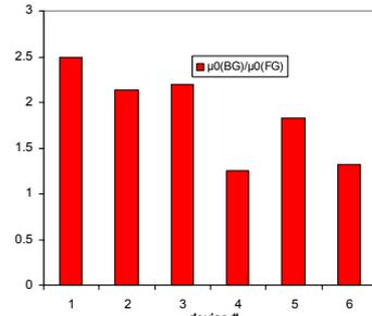
Fig. 8: BG to FG mobility ratio for 100nm DG MOS with oversized BG.
