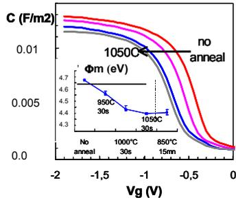
Fig. 7: 2nm  $SiO_2/TiN$  capacitors for 4 thermal budgets (no anneal, 30s at 950, 1000, 1050°C). Insert:  $\Phi_m(TiN)$ .
