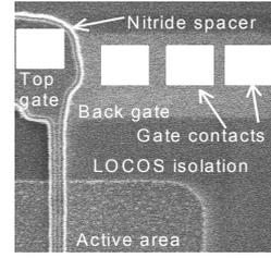
Fig. 3: SEM top view. FG and BG contacts are DUV printed on the ebeam gates (above and below active area).
