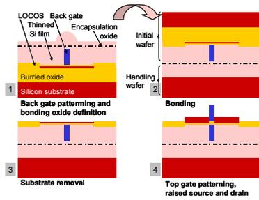
Fig. 1: Process description up to raised source and drain.
