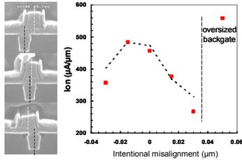
Fig. 4: Left - Misalignment test structures. Right -  $I_{on}$  as a function of intentional misalignment for a 50nm DG MOS (points: experiment, dashed line: simulation).
