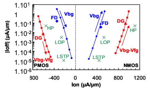
Fig. 14:  $I_{off}$  vs  $I_{on}$  of tunable DG MOS (adjustable  $V_{bg}-V_{fg}$ ) and tunable DG MOS operating in FD mode (adjustable  $V_{bg}$ ) between Low-stand-by-power (LSTP) and High-performance (HP) -90 nm node
