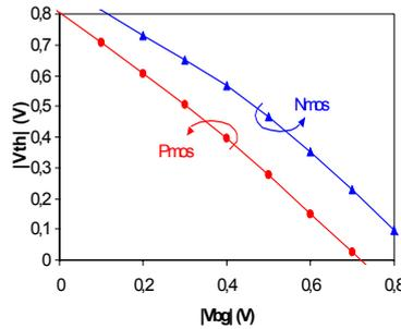
Fig. 13: Tunable threshold voltage of the devices as a function of back gate voltage.
