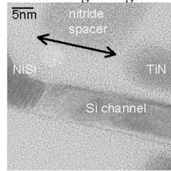
Fig. 5: TEM of NiSi penetration under the spacer and crystalline extension.
