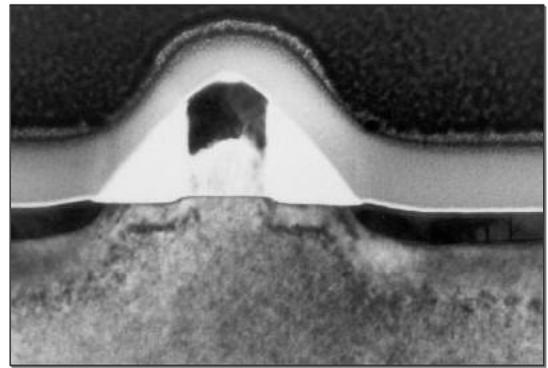
Fig. 1. XTEM of a 50nm transistor with SPER extensions
