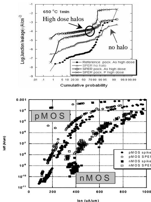
Fig. 2. (a) Area junction leakage for PMOS devices and (b) Ioff vs. Ion curve for NMOS and PMOS SPER devices (open symbols) compared to reference conventional spike devices (closed symbols)
