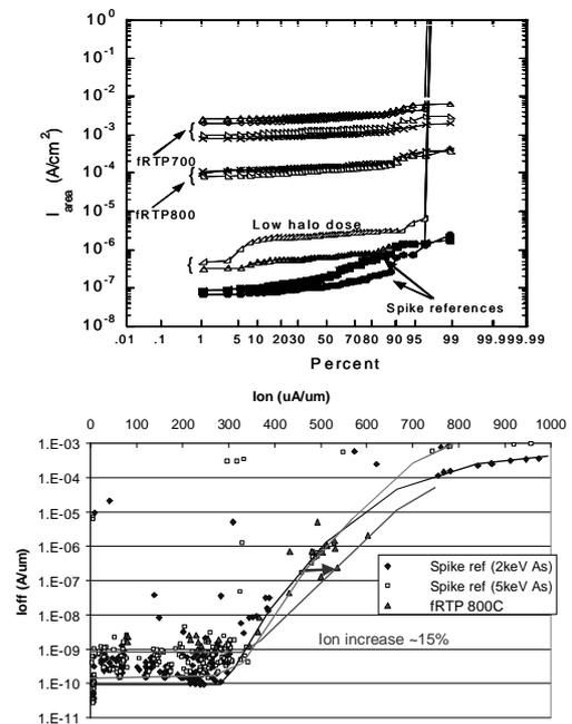
Fig. 3. (a) Area junction leakage and (b) Ioff vs. Ion curve for NMOS fRTP devices compared to reference conventional spike. The intermediate temperature for fRTP is indicated in the figures.
