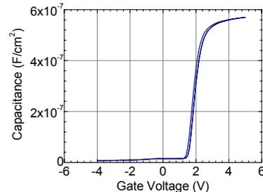
**Fig.3** C-V characteristics of Au/14at.%-YDH/n-Si MIS capacitor. The film was 18.2 nm-thick and annealed at 1000°C. It shows < 50mV hysteresis and a relatively large positive flatband voltage shift. The CET value is determined from the capacitance at V<sub>g</sub> = -5V.
