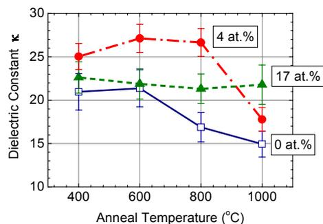
**Fig.5** The relative dielectric constant  $\kappa$  of the Y-doped and undoped  $HfO_2$  films annealed at 400°C, 600°C, 800°C, and 1000°C. The 4at.% doped films show  $\kappa \sim 27$ . The estimated  $\kappa$  decreases severely by the higher temperature annealing in the cases of the undoped and the 4at.% doped film, however, it does not show significant change in the case of 17at.% doped films.
