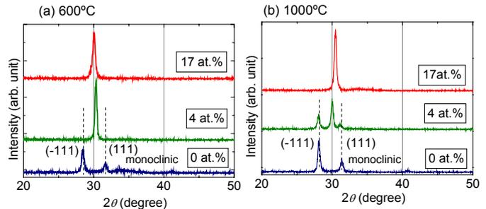
**Fig.1** XRD spectra of Y-doped and undoped HfO<sub>2</sub> films annealed at (a) 600°C and (b) 1000°C. At 600°C, the Y-doped HfO<sub>2</sub> films show a sharp peak around 30° whereas the undoped HfO<sub>2</sub> film shows the peaks corresponding to monoclinic phase structure. The peak around 30° can be assigned to the diffraction from cubic (111), tetragonal (111), or orthorhombic (211). In the case of 4at.% doped film, the monoclinic phase appears at 1000°C by a phase separation.
