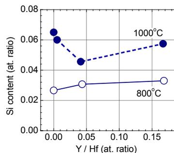
**Fig.6** The amount of Si detected by XPS measured at the film surface. Both the Y-doped and undoped films contain certain amount of Si, although the Y-doped films might slightly restrain the Si diffusion at 1000°C. It suggests that the  $\kappa$  variation with the Y addition (**Fig.5**) is not caused by the Si content difference.
