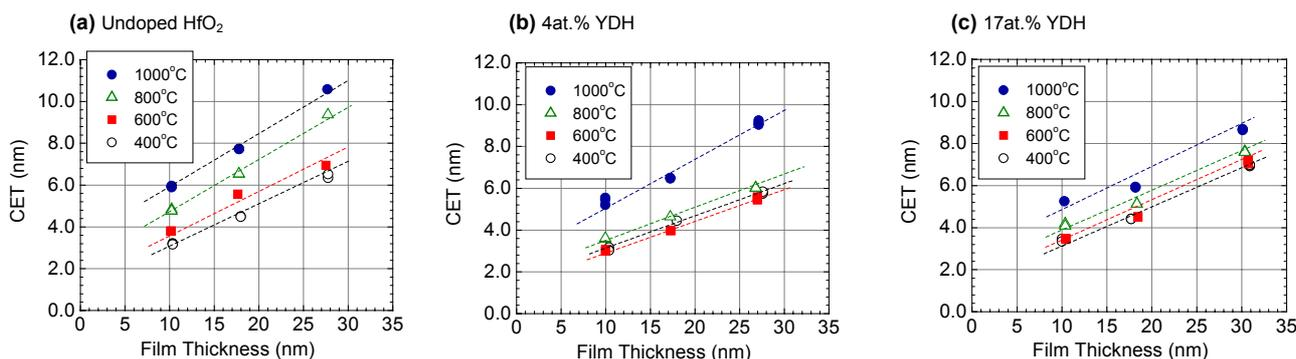
**Fig.4** The relationship between CET and film thickness (determined by GIXR) for (a) undoped film, (b) 4at.% Y-doped film, and (c) 17at.% Y-doped film, annealed at 400°C, 600°C, 800°C, and 1000°C. The dielectric constant ( $\kappa$ ) for each film was estimated from the slope.
