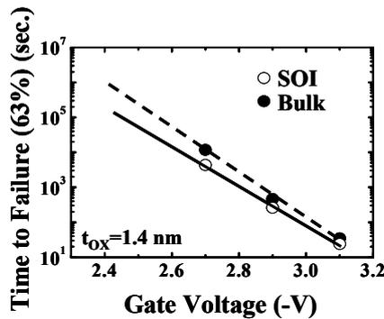
Fig. 8  $t_{fail}$  (63%) vs. stress gate bias for SOI and bulk pMOS devices.
