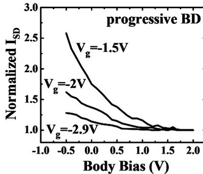
Fig. 6 Body bias dependence of hole current at various gate biases.  $I_{sd}$  is normalized to its value at  $V_b = 2V$ .
