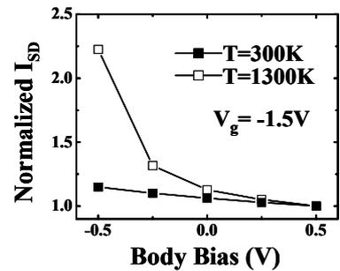
Fig. 10 Simulated body bias effect on hole tunneling current in a 1.4nm oxide pMOS.  $I_{sd}$  is normalized to its value at  $V_b = 0.5V$ .
