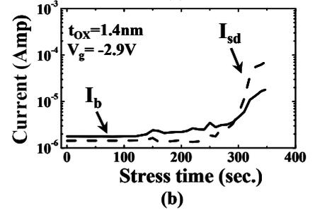
Fig. 4(a) Illustration of current flow in a pMOS at a negative gate bias.  $I_b$  ( $I_{sd}$ ) denotes electron (hole) stress current. (b) Electron and hole current components versus stress time.
