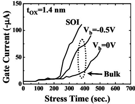
Fig. 2 Oxide breakdown progression in bulk and SOI pMOS. Stress  $V_g = -2.9V$  at  $T=125C$ .
