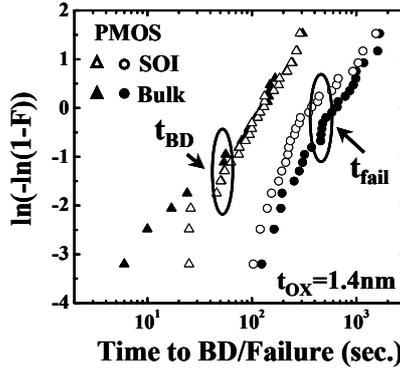
Fig. 3 Weibull plots of  $t_{BD}$  and  $t_{fail}$  distribution for 1.4nm oxide devices.
