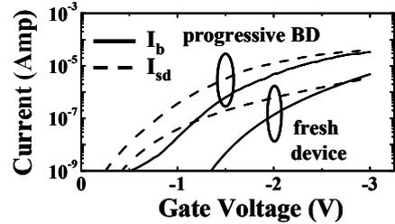
Fig. 7 Gate bias dependence of electron current and hole current in a fresh pMOS and during progressive BD.
