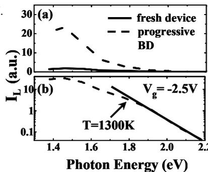
Fig. 9 (a) Spectral distribution of light emission in a 1.4nm oxide pMOS at  $V_g = -2.5V$ . (b) The extracted carrier temperature is around 1300K.
