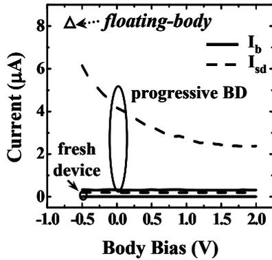
Fig. 5 The dependence of electron current and hole current on body bias at  $V_g = -1.5V$ . Hole current during progressive BD in a floating-body configuration is indicated.
