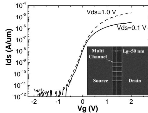
Fig. 7 Current-Voltage characteristics of tri-gate n-MOSFETs (L<sub>g</sub>=50 nm, W<sub>ch</sub>=30 nm) fabricated by ET-PLAD (230°C). Inset shows a SEM image of multi-channel tri-gate n-MOSFETs.
