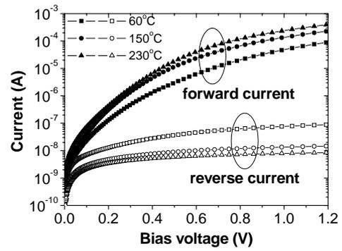
Fig. 5 Current-voltage curves of n<sup>+</sup>-p diode fabricated by ET-PLAD.
