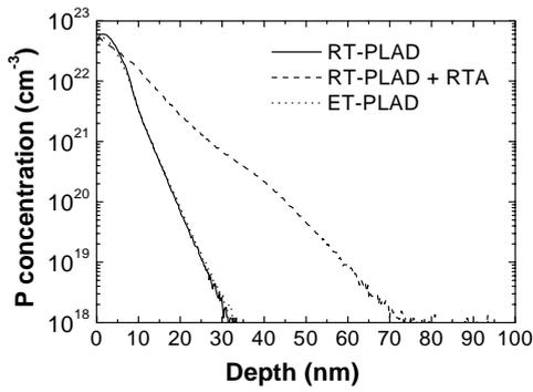
Fig. 1 SIMS depth profiles of phosphorus. RT-PLAD and ET-PLAD were carried out at 27°C and 300°C, respectively. RTA was carried out at 950°C for 30s.
