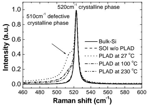
Fig. 3 Raman spectra vs. PLAD temperature.
