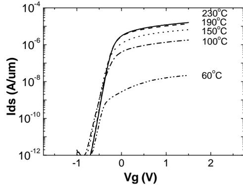
Fig. 6 Subthreshold characteristics of large size SOI n-MOS FETs (L<sub>g</sub>=1 μm, W<sub>ch</sub>=2 μm) as a function of PLAD temperature.
