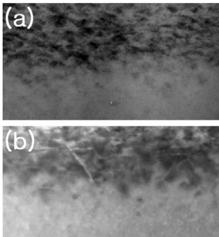
Fig. 4 Cross-sectional TEM images of (a) RT-PLAD and (b) ET-PLAD samples.
