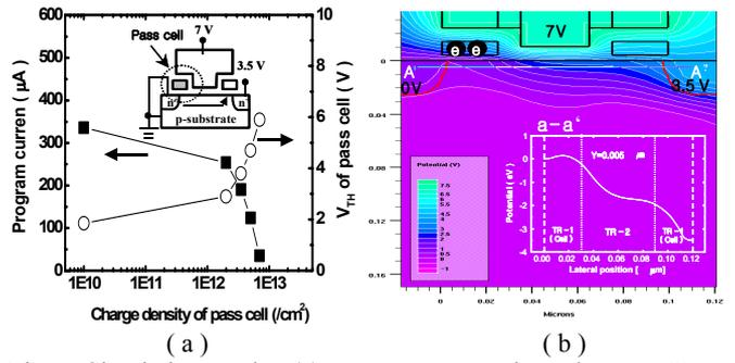
Fig. 5. Simulation results: (a) program current dependence on  $V_{TH}$  of pass cell, (b) channel potential contour across A-A' at the program condition ( $V_{TH}$  of pass cell = 5.9 V)
