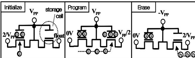
Fig.3 Bias condition for initialization, program and erase. The substrate is grounded.
