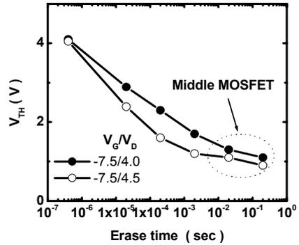
Fig. 7. Over-erase characteristics.  $V_{TH}$  is saturated due to the middle (select) MOSFET without a charge storage node.
