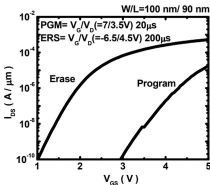
Fig.4  $I_D$ - $V_G$  (@ $V_s = 1.5\text{ V}$ ) characteristics comparison of the split-gate cell after program and erase
