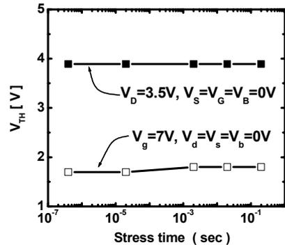
Fig.8 Disturbance from gate and drain for program and erase biasing. Relatively high ONO thickness (3.8/8.5/9.5-nm) suppresses the disturbance.
