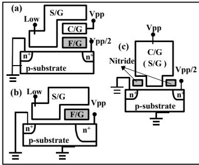
Fig.1 Split-gate flash structures of conventional floating gate (a) triple-gate, (b) source-side injection type, and new (c) SONOS type split-gate
