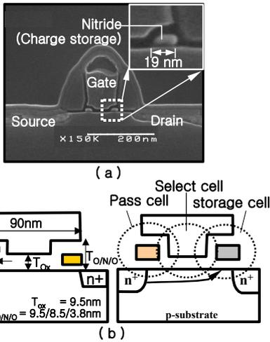
Fig.2 Cross-sectional view: (a) SEM image with self-aligned structure between the gate and storage nitrides (b) schematic diagram. Images of SEM is oxide stained. Thus, Co-silicides on gate and S/D are also stained.
