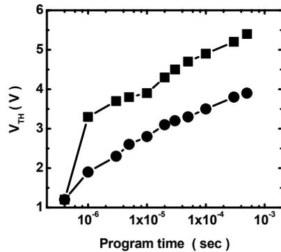
Fig.6 Program speed of split-gate cell; Circle and square symbol marks represent 3V and 4 V  $V_D$ , respectively.  $V_G = 7\text{ V}$  and the others are grounded
