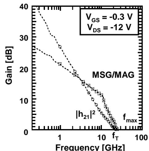
Figure 1. RF gains of 0.2  $\mu$ m gate diamond MISFET.
