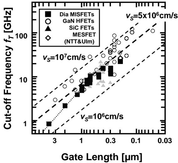
Figure 2. Cut-off frequency of diamond, GaN, SiC transistors as a function of the gate length.
