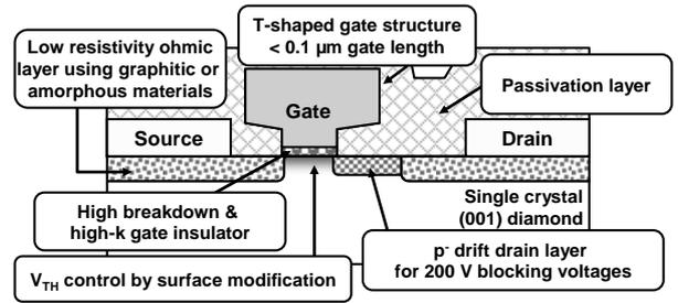
Figure 3. Required device fabrication technology for high power diamond RF transistor.
