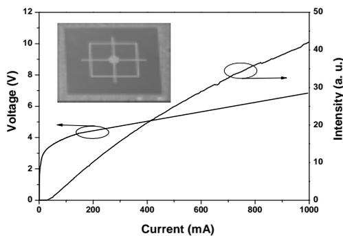
Fig. 3 The L-I-V characteristics of 1×1 mm<sup>2</sup> mesa size LLO-LED. The insertion is the SEM image of the transferred p-side down GaN LED on Cu substrate.
