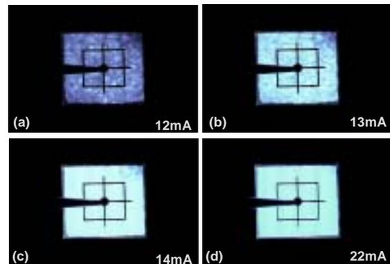
Fig. 3 The emission pictures of the p-side down LLO-LED without transparent contact on it under small operation current, (a) 12mA, (b) 13mA, (c) 14mA and 22mA.
