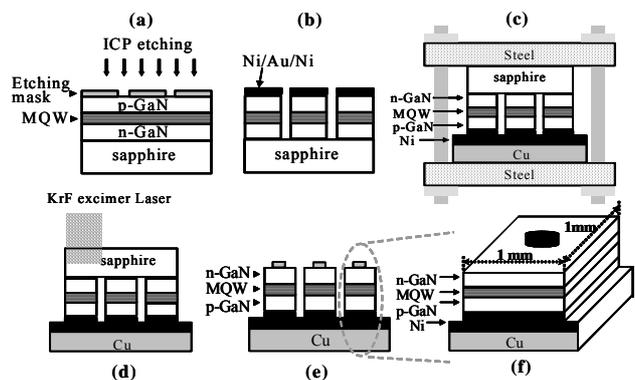
Fig. 1 Fabrication steps of the large-area-emission GaN LEDs with wafer bonding and LLO techniques. (a) Mesa etching by ICP-RIE; (b) Metal deposition; (c) Bonding; (d) Laser lift-off by KrF Laser; (e) n-contact metal deposition; (f) Transferred LED.
