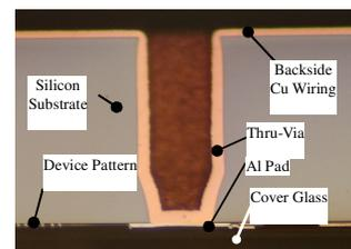
Fig. 3 Cross-sectional micrograph of a thru-via.
