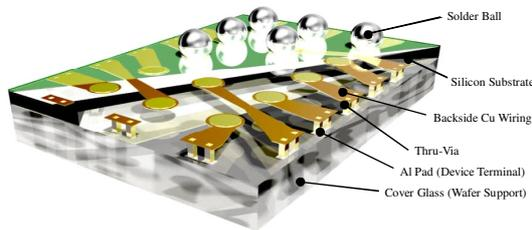
Fig. 1 Structure of image sensor module.
