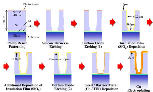
Fig. 2 Process flow diagram of fabricating thru-via.
