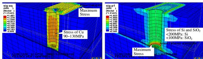
Fig. 4 Structural analysis of a thru-via.
