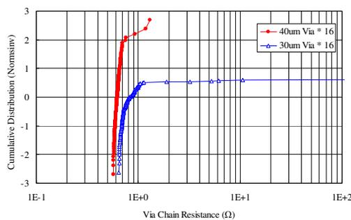
Fig. 5 Thru-via chain resistance within a wafer.
