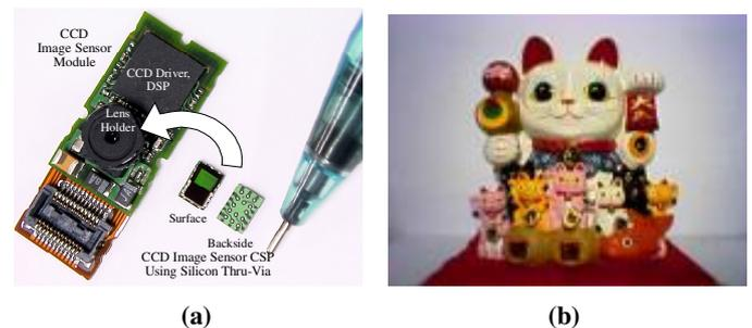
Fig. 6 (a) Image sensor module with thru-via CSP, (b) Photograph taken by the module.
