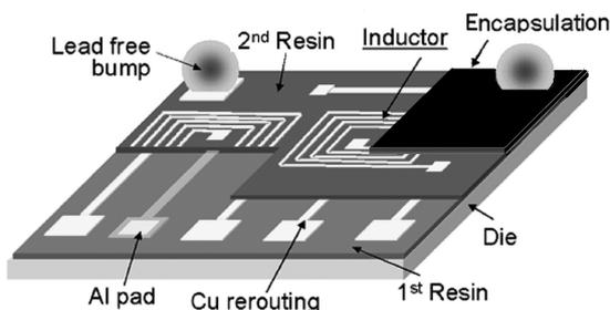
Fig. 1 Schematic illustration of on-chip spiral inductors in WLP.
