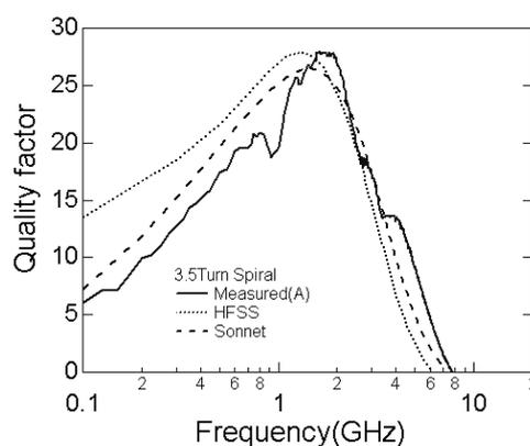
Fig. 4 Comparison between the measured results and simulated values in 3.5 turn spiral inductor with encapsulation layer.
