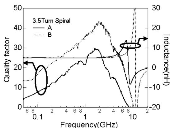
Fig. 3 Frequency dependence of  $L$  and  $Q$  in 3.5 turn spiral inductors without encapsulation layer.
