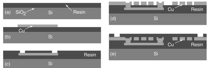
Fig. 2 Schematic cross-sectional diagram of the fabrication process. (a) Resin coating and curing (b) Formation of bottom conductive layer by Cu electroplating (c) Photosensitive resin coating, patterning and curing (d) Formation of upper conductive layer including coil patterns, grounds pattern and test pads by Cu electroplating. (e) Encapsulation resin coating.
