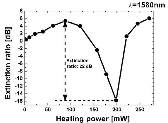
Fig. 3 The switching characteristics of PC optical switch.
