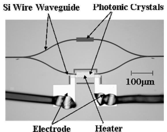
Fig. 2, Microscopic view of fabricated PhC optical switch.
