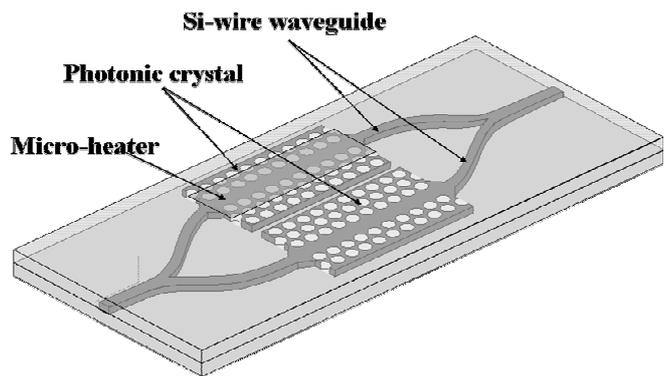
Fig. 1, Structure of fabricated PhC optical switch.
