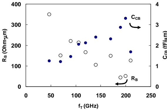
Figure 2. Base resistance  $R_B$  (open symbols) and collector-base capacitance  $C_{CB}$  (solid symbols) for reported SiGe HBTs. Values are normalized to emitter length [3,4,6-11].
