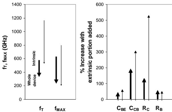
Figure 3. Electrical parameter shifts with addition of the device extrinsic portion as predicted by TCAD simulation. Thick arrows are the 350GHz device as reported in [14]; Thinner arrows are simulated 1.16 THz (intrinsic) device.
