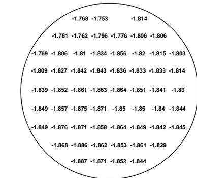
Fig. 8.  $V_{th}$  Distribution of GaN-HEMT fabricated on a 3-inch S.I.-SiC substrate. Standard deviation was 34 mV.
