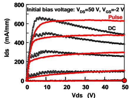
Fig. 3. DC and Pulsed I-V characteristics. Bias point of pulsed measurements was  $V_{ds}$  of 50 V and  $V_{gs}$  of -2 V. Pulse period and pulse duration are 1 ms and 1  $\mu\text{s}$ , respectively.
