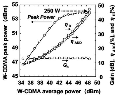
Fig. 5. Power characteristics of a 250 W push-pull amplifier at W-CDMA modulation scheme of  $V_{ds}$ =50 V.
