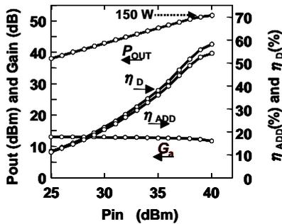
Fig. 4. Measurement of a 150 W CW power of single-chip Al-GaN/GaN HEMT amplifier at 2.1 GHz. Quiescent drain current was 500 mA at  $V_{ds}$ =63 V.
