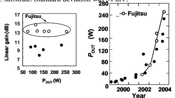
Fig. 9. Linear gain and power trend of GaN-HEMTs.
