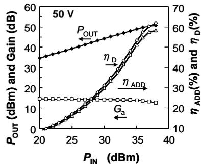
Fig. 6. Power characteristics of a 14.5-dB-gain 116 W amplifier.
