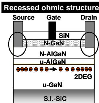
Fig. 1. Schematic cross-sectional view of AlGaIn/GaN HEMT with surface-charge-controlled n-GaN-cap structure.
