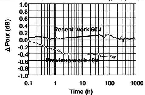
Fig. 7. Power characteristics under P3dB RF-stress test at 30, 40, and 60 V.
