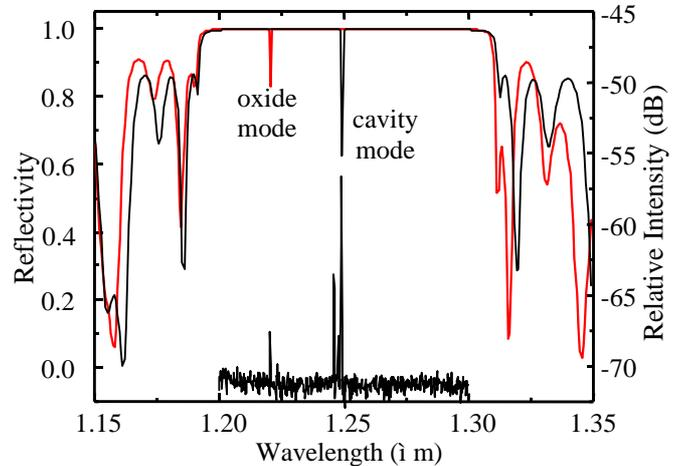
Fig. 5 Simulated reflectance spectra of oxidized and unoxidized sample F with a 12 mA driving current. Lasing spectrum of sample F was also plotted.
