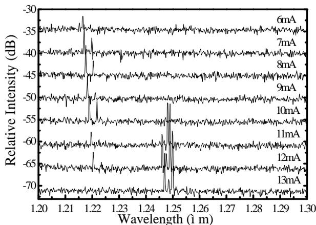
Fig. 4 Lasing spectra of sample F with various driving currents.
