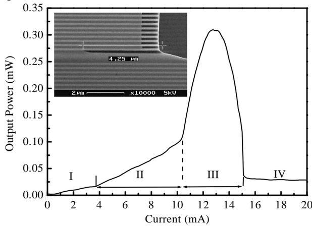
Fig. 3 A more detailed L-I characteristics of sample F. Inset shows SEM picture of the oxidized layers.
