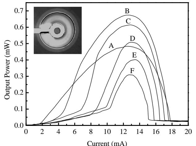
Fig. 2 L-I characteristics for these six devices. Inset shows top view of the fabricated VCSELs.
