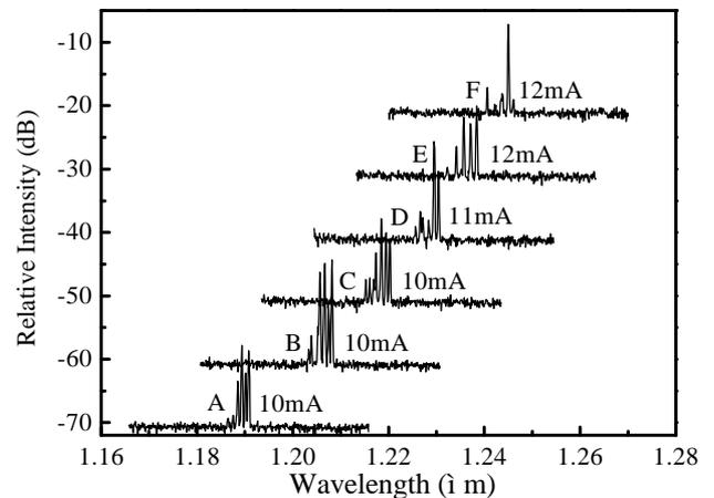
Fig. 1 Lasing spectra of the six VCSELs measured near thermal rollover.
