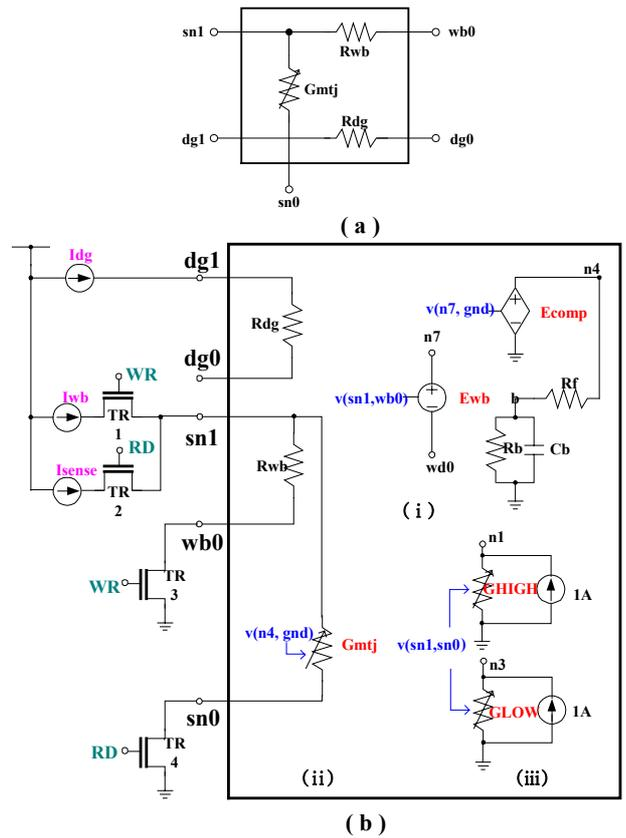
Fig. 2. (a) Block diagram and (b) schematic of macro-model for MTJ.
