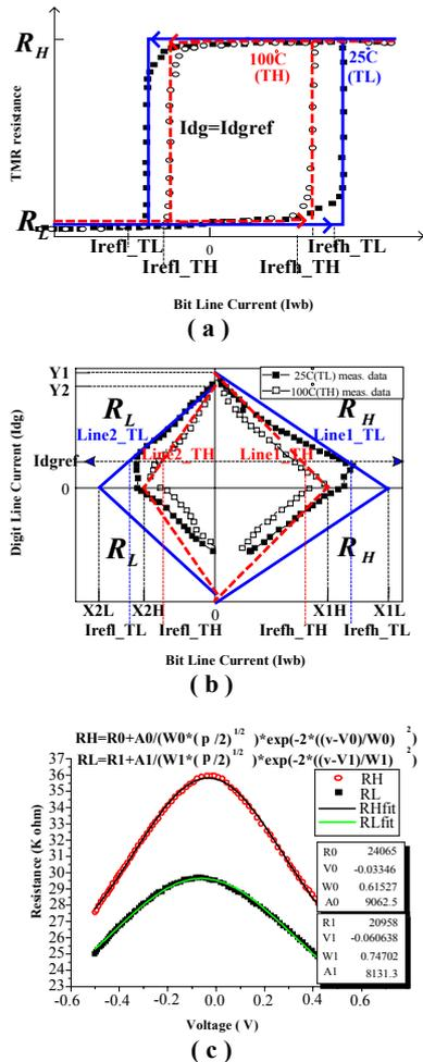
Fig. 1. (a) Hysteresis and (b) asteroid curves at 25°C and 100°C (symbols: measured data, lines: simple fitting line), (c) R-V characteristics (symbols: measured data, lines: gaussian fitting data).
