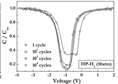
**Fig 8.** QSCV curves of SONOS devices annealed in HP-H<sub>2</sub> (10atm) as a function of P/E cycles.
