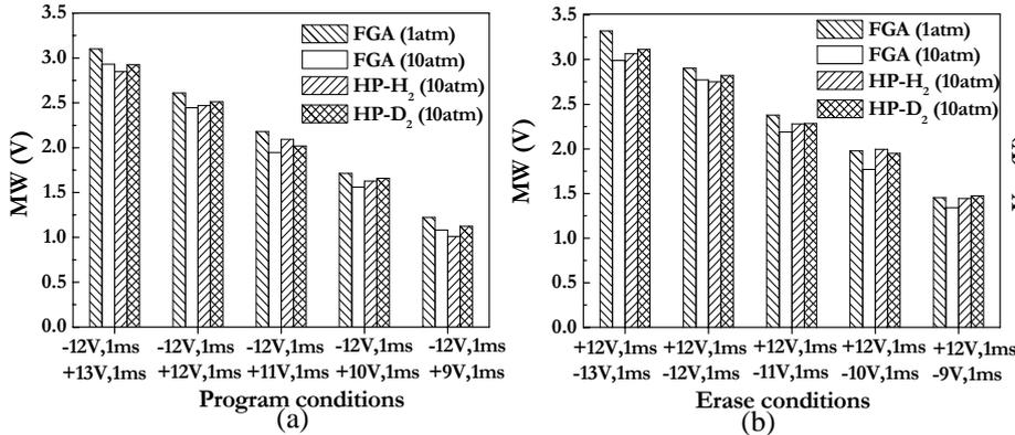
**Fig 1.** (a) Program and (b) erase characteristics of fabricated SONOS devices annealed in each ambient.
