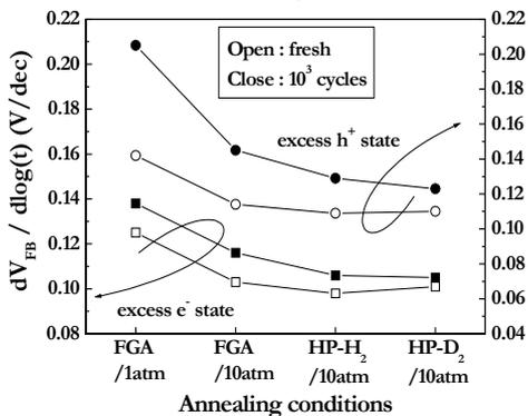
**Fig 9.** Charge decay rate of fabricated SONOS devices annealed in each ambient.
