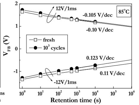
**Fig 2.** Retention Characteristics of SONOS devices annealed in HP-D<sub>2</sub> (10atm).
