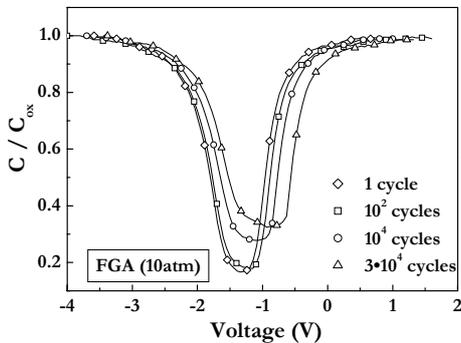
**Fig 6.** QSCV curves of SONOS devices annealed in FG (10atm) as a function of P/E cycles.
