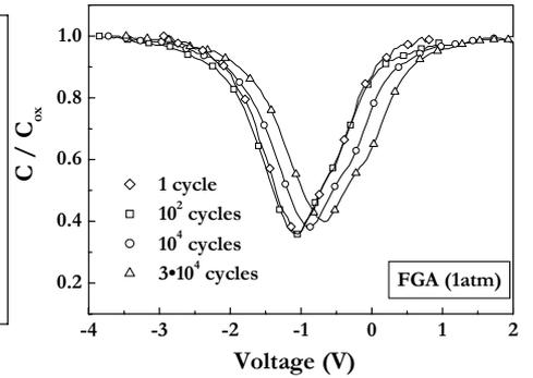
**Fig 5.** QSCV curves of SONOS devices annealed in FG (1atm) as a function of P/E cycles.
