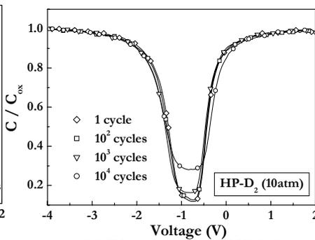
**Fig 7.** QSCV curves of SONOS devices annealed in HP-D<sub>2</sub> (10atm) as a function of P/E cycles.
