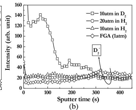
**Fig 10.** SIMS depth profiles of ONO stack annealed in H<sub>2</sub> or D<sub>2</sub> ambients. (a) Hydrogen profiles, (b) Deuterium profiles.
