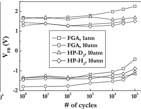
**Fig 4.** Endurance characteristics of SONOS devices.
