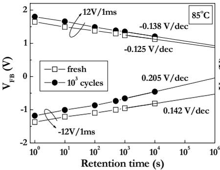
**Fig 3.** Retention Characteristics of SONOS devices annealed in FG (1atm).
