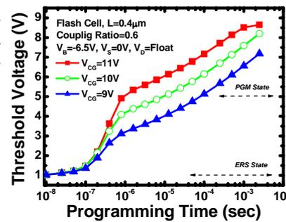
Fig. 7  $V_t$  shift as a function of programming time for different control gate voltages.
