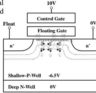
Fig. 1 Cell structure and schematic illustration of hot electron generation by BBISHE mechanism
