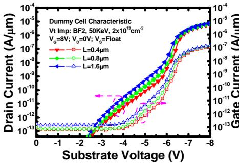
Fig. 6 The measured current spectrums with the different channel length.
