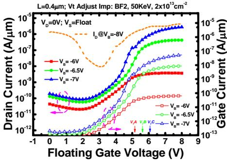
Fig. 3 The measured current spectrums with the different floating gate voltages.
