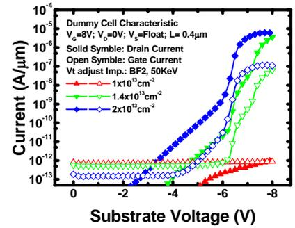
Fig. 5 The measured current spectrums with the different  $V_t$  adjust implantation splits.
