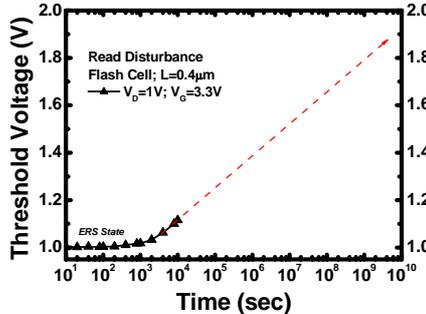
Fig. 10 The 10 years lifetime prediction of read disturbance characteristics.
