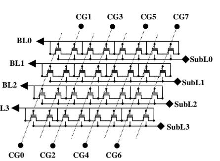
Fig. 2 Array architecture and the illustration of hot electron generation by selective p- sub lines divided by STI
