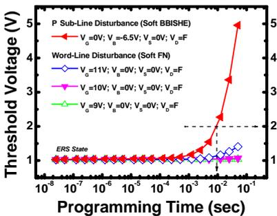
Fig. 9 The measured sub-line and word-line disturbance characteristics
