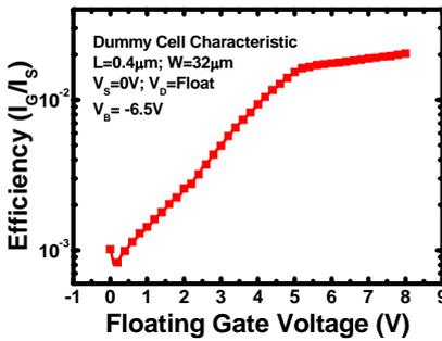
Fig. 4 The measured efficiency ( $I_G/I_S$ ) of dummy cell during programming operation.
