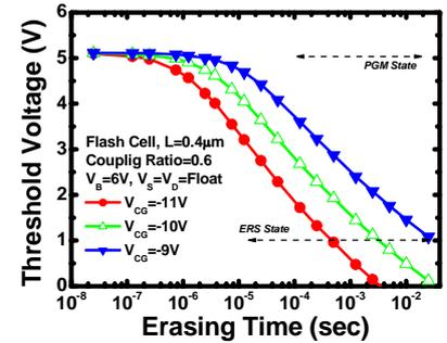
Fig. 8  $V_t$  shift as a function of erasing time for different control gate voltages.
