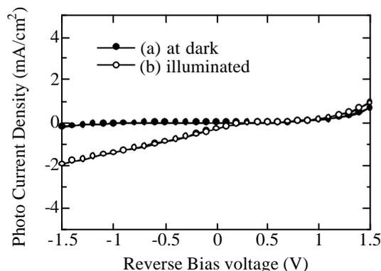
Fig. 3. Current-voltage characteristics of ITO / CuPc (20nm) / BPPC (20nm) / a-C:N / ITO with active area of 0.1mm<sup>2</sup>. The red LED for illumination has emission peak at about 640nm.
