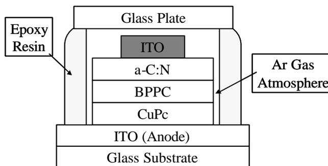
Fig. 2. A schematic of typical photo detector.
