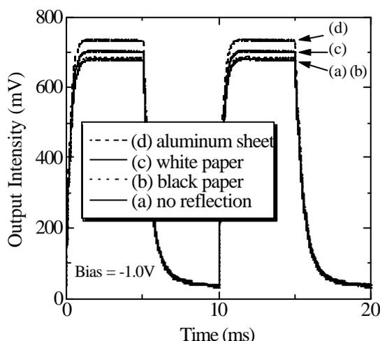
Fig. 4 Photo response dependence of the output current intensity with reflection of a black or white sheet and an aluminum sheet at -1.0V bias voltage at 100Hz modulation. 100kΩ terminal resistance was used for measuring the output current.
