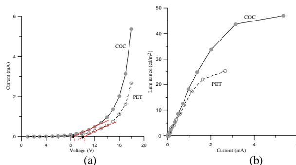
Fig. 3(a) Voltage-Current characteristics of an OLED with COC and PET substrate, where 1 and 2 represent the turn-on voltage of the COC (8.4V) and PET (10.0V), respectively; (b) Current-Luminance characteristics of an OLED with COC (45cd/m<sup>2</sup>) and PET (23cd/m<sup>2</sup>) substrate.
