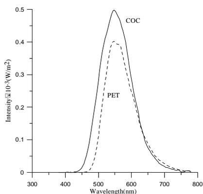
Fig. 4 Electroluminescence spectra of an OLED with COC and PET substrates.
