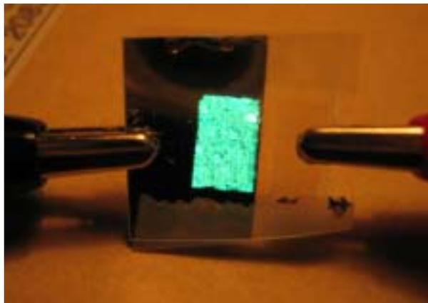
Fig. 6 Photo image of a FOLED in bending with a configuration of COC substrate/ITO/ NPB/Alq<sub>3</sub>/LiF/Al.
