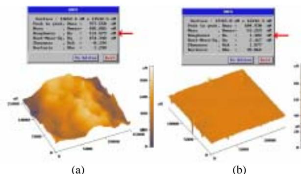
Fig. 2 AFM images for COC substrate (a) before annealing and (b) after annealing.
