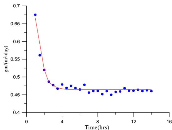
Fig. 1 H<sub>2</sub>O permeation rate curve of the COC substrate at 25°C.
