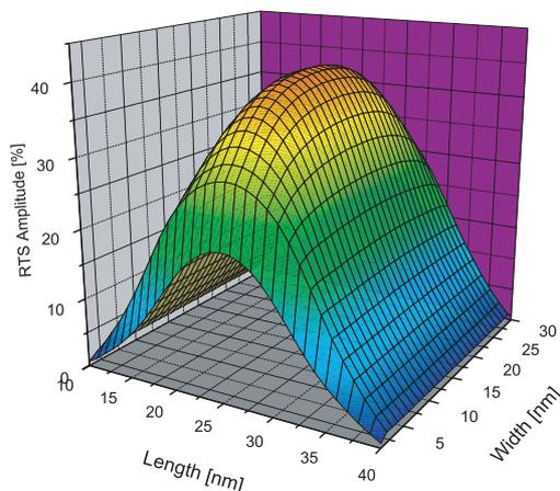
Figure 1. Dependence on trap position within the channel of RTS fluctuations in the drain current of a 30×30nm MOSFET.
