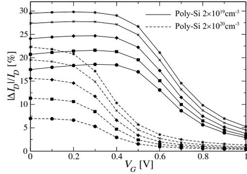
Figure 6. Relative RTS amplitudes for a 30 nm n-channel MOSFET with high- $\kappa$  dielectric thickness,  $t_{ox}=5.64\text{nm}$ , for a trap at different positions within the oxide. Two different dopings of poly-Si gate are shown.
