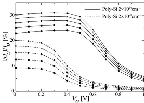
Figure 5. Relative RTS amplitudes for a 30 nm n-channel MOSFET with oxide thickness,  $t_{ox}=1\text{nm}$ , for a trap at different positions within the oxide. Two different dopings of poly-Si gate are shown.
