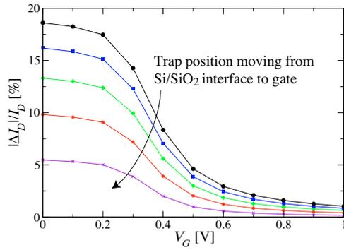
Figure 4. Relative RTS amplitudes for a 30 nm n-channel MOSFET with oxide thickness,  $t_{ox}=1\text{nm}$ , for a trap at different positions within the oxide. A metal gate is assumed.
