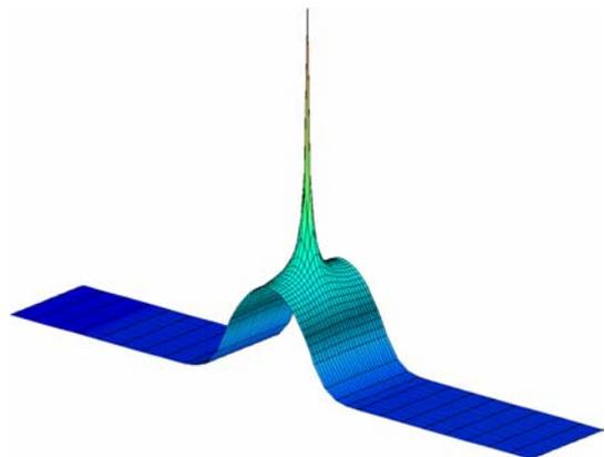
Figure 2. The potential barrier between source and drain in a MOSFET, and the effect on this of a single trapped electron in the centre of the channel located at the Si/SiO<sub>2</sub> interface.
