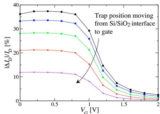
Figure 3. Relative RTS amplitudes for a 30 nm n-channel MOSFET with oxide thickness,  $t_{ox}=3\text{nm}$ , for a trap at different positions within the oxide. A metal gate is assumed.
