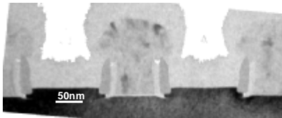
Figure 4. TEM cross-section of raised source/drain architecture for optimized SEG process in sequence B.
