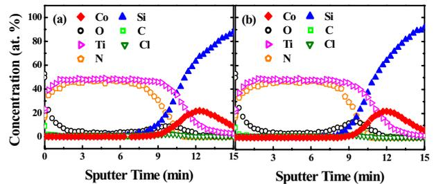
Fig. 5. AES analysis of CVD-Co/CVD-Ti/TiN/680°C, 7hr silicide morphology on (a) n+ Si (b) p+ Si
