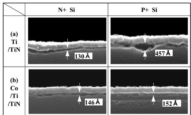
Fig. 6. SEM images of CVD-Co and CVD-Ti silicide morphology/(on n+/p+ Si) (a) CVD-Ti/TiN (b) CVD-Co/CVD-Ti/TiN
