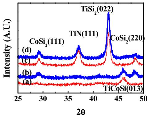
Fig. 3. XRD analysis of CVD-Ti/TiN after CVD-Co deposition for a) n+ Si/CVD-Co/CVD-Ti b) p+ Si/CVD-Co/CVD-Ti c) n+ Si/CVD-Co/CVD-Ti/TiN with thermal budget and d) p+ Si/CVD-Co/CVD-Ti/TiN with thermal budget
