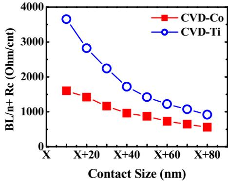
Fig. 1. Contact resistance of CVD-Co and CVD-Ti silicide on BL/n+ Si with various contact size.
