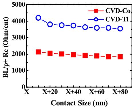
Fig. 2. Contact resistance of CVD-Co and CVD-Ti silicide on BL/p+ Si with various contact size.
