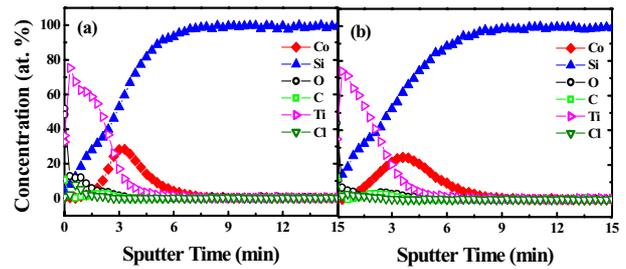
Fig. 4. AES analysis of CVD-Co/CVD-Ti silicide morphology on (a) n+ Si (b) p+ Si
