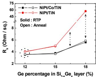
Fig. 6 sheet resistance according to Ge percentages in  $Si_{1-x}Ge_x$  before and after the post-silicidation annealing at 600 °C for 30 min.
