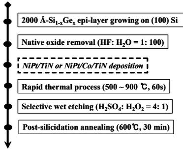
Fig. 1 The process flow.
