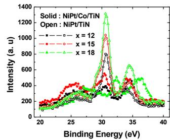
Fig. 8 XPS surface binding energies of Ge in case with- and without the Co over-layer.
