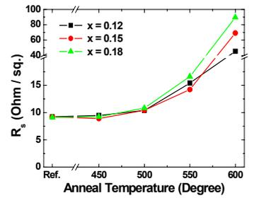
Fig. 3 Sheet resistance in case the pure-Ni according to the annealing temperature.
