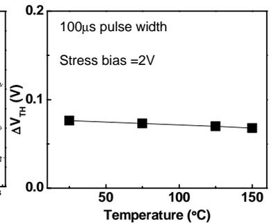
Fig. 7 Dependence of the stress-induced ΔV<sub>TH</sub> on the stress temperature
