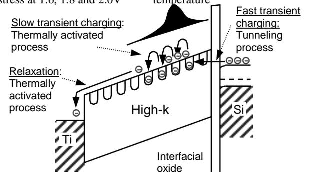
Fig. 10 Schematic of the electron trapping and redistribution processes. Fast transient charging is associated with the resonance electron tunneling into the traps. While the thermally activated charge redistribution process may contribute during long stresses
