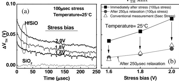
Fig. 5 (a) Post-stress time dependence of the V<sub>TH</sub> shift induced by the 100µsec stress at V<sub>g</sub>=1.6V, 1.8V and 2.0V (b) V<sub>TH</sub> shift immediately after the 100µsec stress and after 250µsec post-stress relaxation period vs. stress voltage. Open symbols represent V<sub>TH</sub> shift after 5sec stress measured using conventional I<sub>D</sub>-V<sub>g</sub> method
