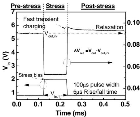
Fig. 3 Typical V<sub>in</sub> and V<sub>out</sub> signals of the inversion pulse measurement
