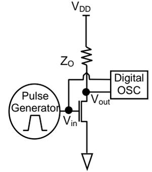
Fig. 2 Diagram of the inversion pulse measurement [9]
