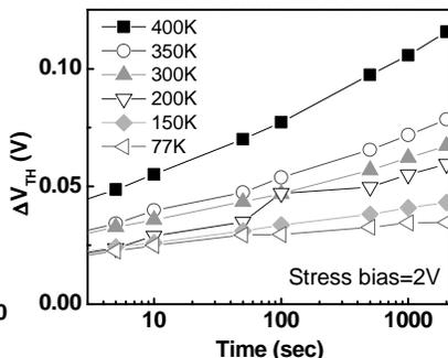
Fig. 9 Stress time dependence of the V<sub>TH</sub> shift at different stress temperatures
