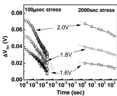
Fig. 6 Post-stress time dependence of V<sub>TH</sub> shift induced by 100µsec and 2000sec stress at 1.6, 1.8 and 2.0V
