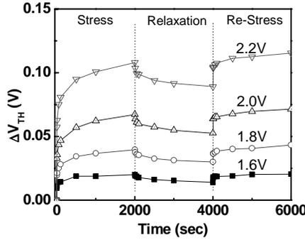
Fig. 1 Time dependence of V<sub>TH</sub> values during stress with V<sub>g</sub>= 1.6V to 2.2V and relaxation at V<sub>g</sub>=0V
