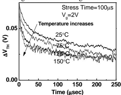
Fig. 8 Post-stress time dependence of the V<sub>TH</sub> shift at different temperatures
