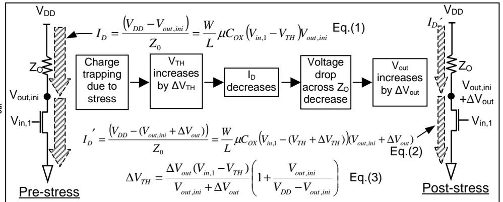
Fig. 4 Schematic for the V<sub>out</sub> change during inversion pulse measurements and the calculation of the V<sub>TH</sub> shift
