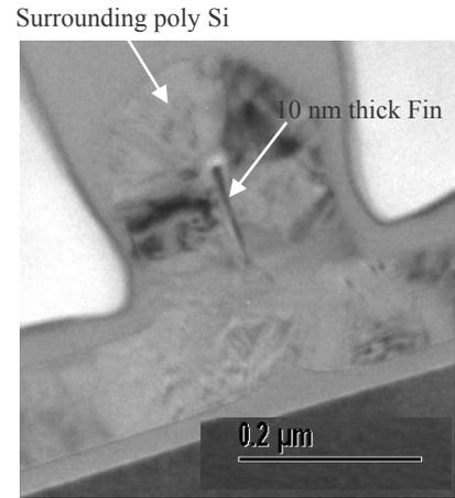
**Fig. 3** TEM image of an ultra narrow (~10 nm thick), 100 nm tall silicon fin after gate  $\alpha$ -silicon deposition. The fin is fully wrapped in side the  $\alpha$ -Si showing a true GAA structure.
