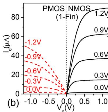
**Fig. 4** I-V characteristics of ~10 nm thick, 100 nm long and 100 nm tall silicon body GAA transistors. (a)  $I_d$ - $V_g$  plots (b)  $I_d$ - $V_d$  plots – the number shown in volts with each curve is gate overdrive ( $V_g$ - $V_{th}$ ). For both the plots, the currents are per device.
