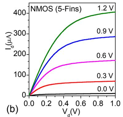
**Fig. 7** I-V characteristics of five ~10 nm thick, 100 nm long and 100 nm tall lateral Si-fins GAA n-FET (a)  $I_d$ - $V_g$  plots (b)  $I_d$ - $V_d$  plots - the number shown in volts with each curve is gate overdrive ( $V_g$ - $V_{th}$ ). For both the plots, the currents are per device.
