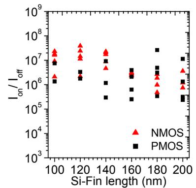
**Fig. 5** Effect of fin length of GAA NMOS and PMOS transistors on  $I_{on}/I_{off}$ .
