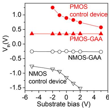
**Fig. 6** Effect of substrate bias on GAA n- and p-FET devices with a comparison to control devices.
