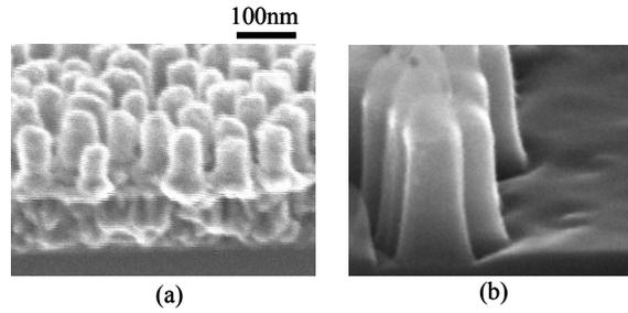
Fig. 5. SEM images for (a) nickel mask rods (b) silicon pillars along the edge of active region.
