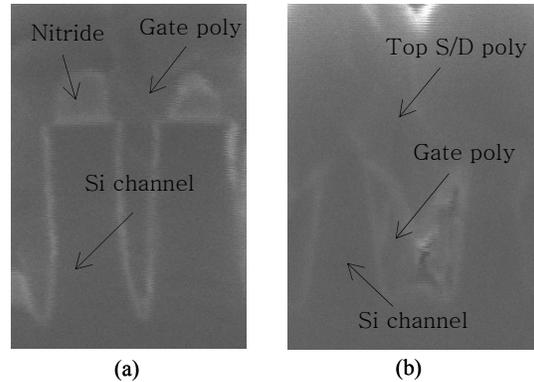
Fig. 6. SEM images for (a) silicon pillars after gate poly deposition (b) final transistor structure.
