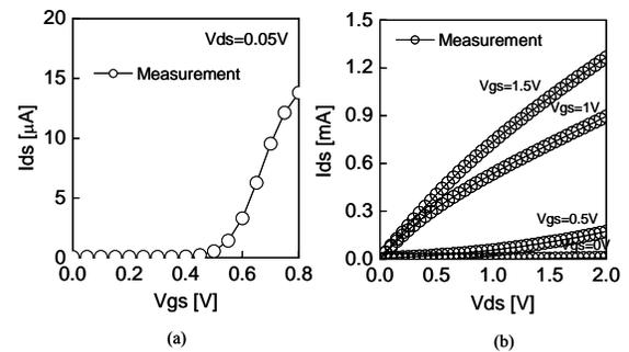
Fig. 7. Electrical characteristics of the device (a)  $I_{ds}$ - $V_{gs}$  curve (b)  $I_{ds}$ - $V_{ds}$  curve.
