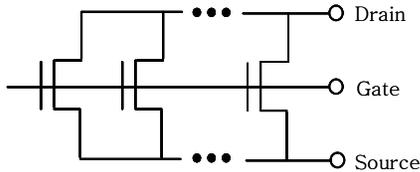
Fig. 2. Equivalent circuit of the transistor with multi-pillar silicon channels.
