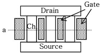
Fig. 1. Schematic diagram of the transistor with multi-pillar silicon channels.
