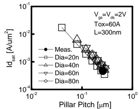
Fig. 8. Relationship between the drain current and the pillar pitch for different silicon pillar diameters.
