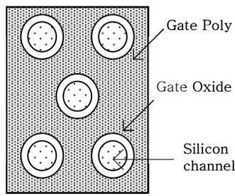
Fig. 3. Plane view of the transistor along a-a' cross-section of Fig. 1.
