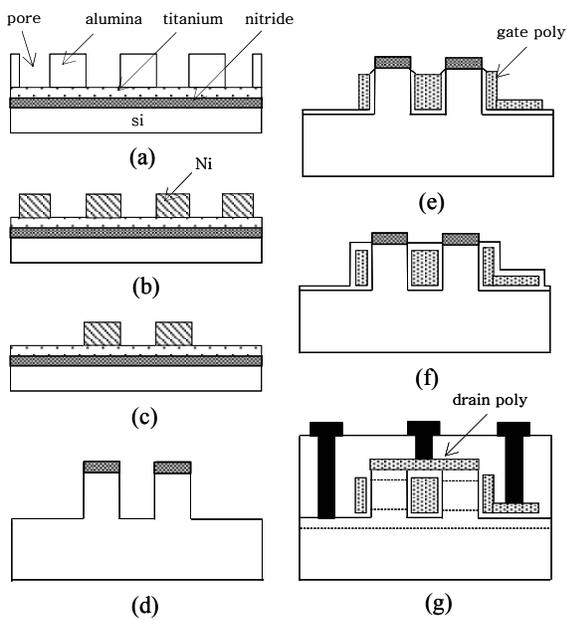
Fig. 4. Process sequence of the transistor with multi-pillar silicon channels.
