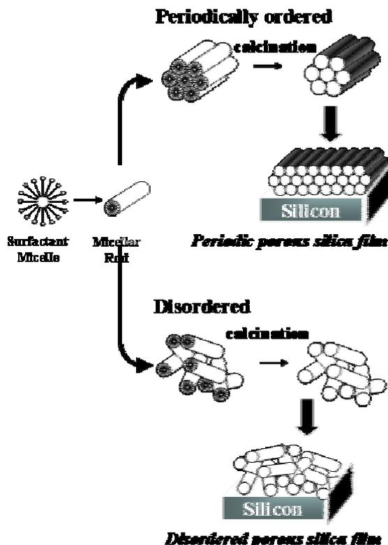
Fig. 2 Schematic diagram of preparation of disordered or periodically ordered porous silica films [2].
