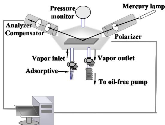
Fig.1 Schematic diagram of the measurement setup
