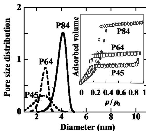
Fig.5 Isotherms (inset) and pore size distributions of disordered porous silica films prepared with templates P45, P64, P84.
