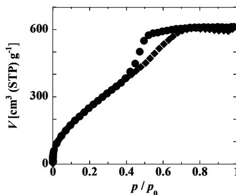
Fig. 4 Argon adsorption / desorption isotherm of disordered porous silica film with  $C_t = 1$ .
