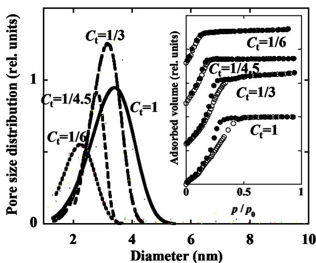
Fig.3 Adsorption / desorption isotherms (inset) and pore size distributions of disordered porous silica films prepared with varied P45 template concentrations.
