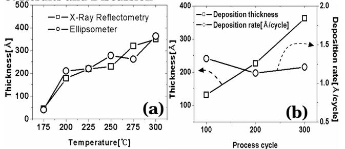
Fig. 2 ALD temperature window and deposition rate by X-ray reflectometry and ellipsometer.
