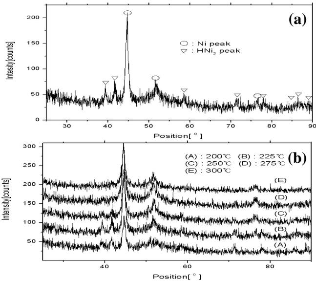
Fig. 4 Composition measurement of XRD deposited Ni thin film.
