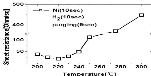
Fig. 3 Sheet resistance measurement by 4-point probe.
