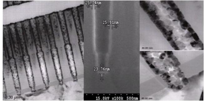
Fig. 5 Cross sectional TEM and SEM images of the deposited Ni film in the trench with aspect ratio of 1:16.
