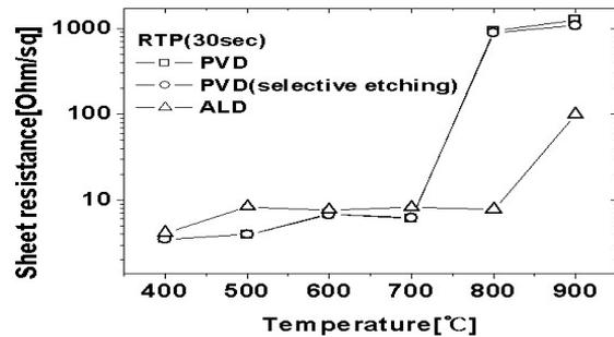
Fig. 6 Sheet resistance Ni-silicide after RTP process at temperatures from 400°C to 900°C.
