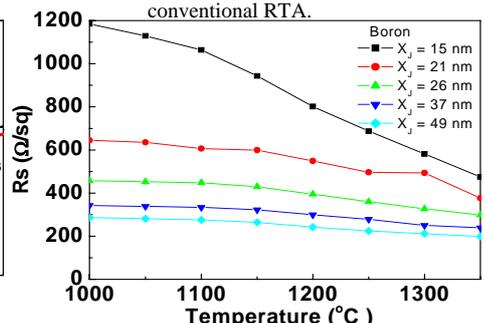
Fig. 15. Calculated plot of R<sub>s</sub> vs. temperature of diffusion-less annealing process.
