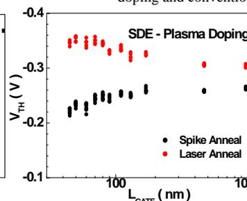
Fig. 10. Comparison of V<sub>TH</sub> roll off of laser annealing with conventional RTA.
