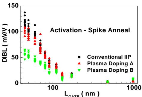
Fig. 6. DIBL characteristics of plasma doping and conventional ion implantation.
