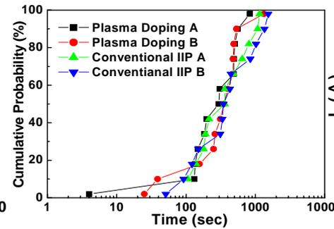
Fig. 7. Gate oxide QBD distributions of plasma doping and conventional ion implantation process.
