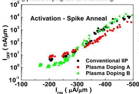
Fig. 4. I<sub>ON</sub>-I<sub>OFF</sub> correlation of conventional ion implantation and plasma doping.
