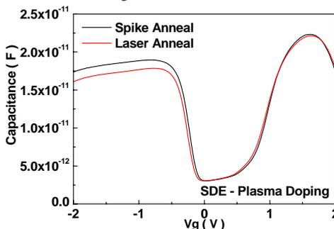
Fig. 13. PMOS C-V characteristics of laser annealing vs. conventional RTA.
