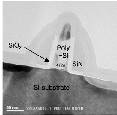
Fig. 2. Cross sectional TEM image of sub 50 nm gate length PMOSFET.
