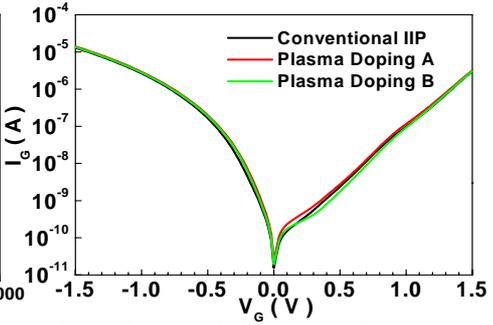
Fig. 8. Gate oxide leakage current characteristics of ion implantation and plasma doping process.
