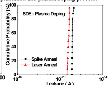
Fig. 12. Junction leakage current distribution of laser annealing and conventional RTA.
