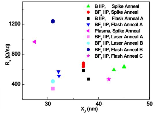
Fig. 3. X<sub>j</sub>-R<sub>s</sub> plot with various ion implantations, plasma doping, and annealing processes.
