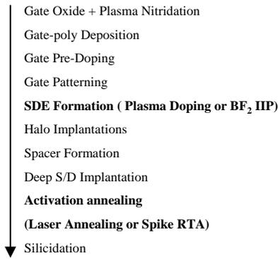
Fig. 1. Process flow of transistor fabrication using plasma doping and laser annealing.
