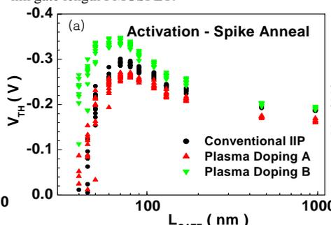
Fig. 5. (a) Low V<sub>TH</sub> PMOSFET V<sub>TH</sub> roll-off and (b) High V<sub>TH</sub> PMOSFET V<sub>TH</sub> roll-off comparison of conventional ion implantation with plasma doping.
