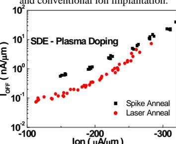
Fig. 9. Comparison of I<sub>ON</sub>-I<sub>OFF</sub> correlation of laser annealing with conventional RTA.
