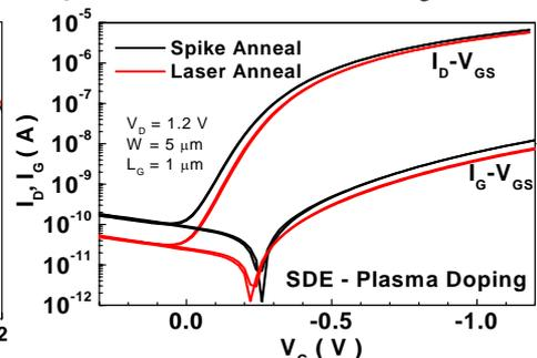
Fig. 14. I<sub>D</sub>-V<sub>GS</sub>, I<sub>G</sub>-V<sub>GS</sub> plot of laser annealing and spike annealing. L<sub>GATE</sub>=1.0 μm.
