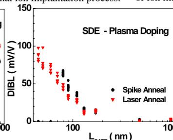
Fig. 11. DIBL comparison of laser annealing with conventional RTA.
