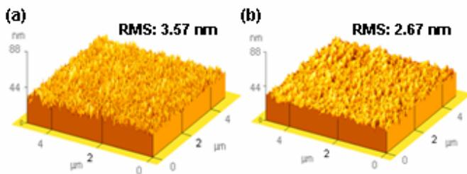
Fig. 5. Three-dimensional AFM surface morphologies (a) 50 nm-SiO<sub>x</sub> (b) 150 nm-parylene/50 nm-SiO<sub>x</sub> on PC substrate.
