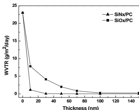
Fig.1. WVTR of PECVD SiN<sub>x</sub> and SiO<sub>x</sub> films on PC substrates as a function of film thickness.
