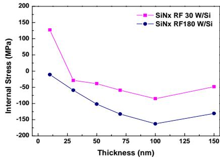
Fig. 2. Internal stress of SiN<sub>x</sub> deposited on Si wafer as a function of film thickness.
