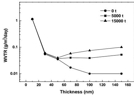
Fig. 3. WVTR of SiN<sub>x</sub> film on PC substrates bended for 0, 5000 and 15000 times as a function of film thickness.
