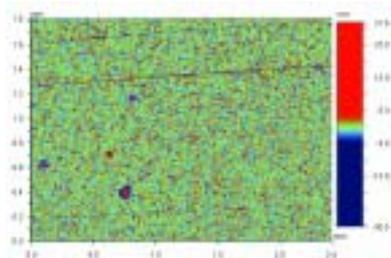
Fig. 6. Two-dimensional surface morphologies of 50 nm-SiO<sub>x</sub> film on PC substrates.
