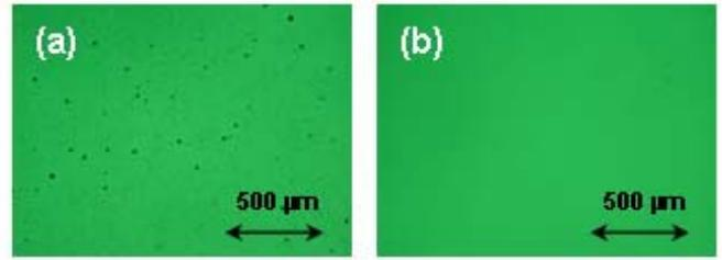
Fig. 7. Comparison of emission characteristics of (a) single PON and (b) double PON layers capped OLEDs after 100 h under 25°C, 40%RH.
