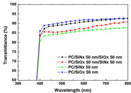
Fig. 4. Transmittance of SiN<sub>x</sub>, SiO<sub>x</sub>, SiN<sub>x</sub>/SiO<sub>x</sub> and SiO<sub>x</sub>/SiN<sub>x</sub> on PC substrates as a function of wavelength.
